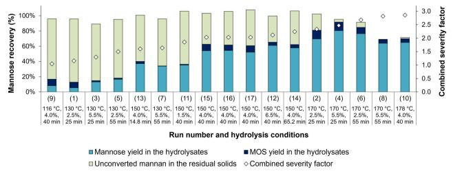
Fig. 2 Mannose mass balances in the hydrolysates and residual solids after dilute-oxalic acid hydrolysis of açaí seeds. Mannose recoveries include mannose and MOS yields in the hydrolysates and unconverted mannan in the residual solids, all expressed as a percentage of the total mannose potential of in natura seeds.
