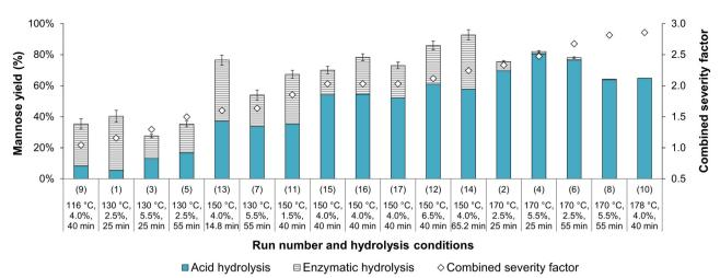
Fig. 4 Mannose yield in the dilute oxalic acid hydrolysis and subsequent enzymatic hydrolysis of açaí seeds, expressed as a percentage of the total mannose potential of *in natura* seeds ( $Y_{1/0}$  in blue,  $Y_{2/0}$  in dashed gray).
