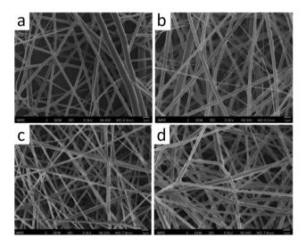
Fig. 23 SEM images of electrospun (a) PCL, (b) PCL/LP1, (c) PLLA, and (d) PLLA/LP1 nanofibers. Scale bars = 1  $\mu$ m. Reproduced from ref. 143 with permission from American Chemical Society, copyright 2017.
