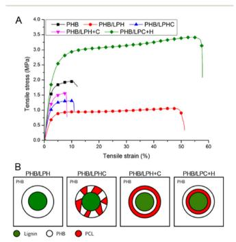
Fig. 25 (A) Typical stress-strain curves of electrospun nanofibers obtained from a tensile test. (B) Proposed dispersion models to show how different lignin copolymers disperse in PHB matrix. Reproduced from ref. 156 with permission from Elsevier, copyright 2018.
