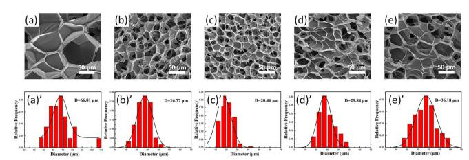
Fig. 11 (a)—(e) SEM images of cell morphology; (a)'—(e)' corresponding cell size distributions of the PLA and PLA/lignin-*graft*-PLA foams: (a) and (a)' neat PLA, (b) and (b)' 1 wt% lignin-*graft*-PLA, (c) and (c)' 3 wt% lignin-*graft*-PLA, (d) and (d)' 5 wt% lignin-*graft*-PLA, and (e) and (e)' 7 wt% lignin-*graft*-PLA. Reproduced from ref. 111 with permission from John Wiley and Sons, copyright 2020.
