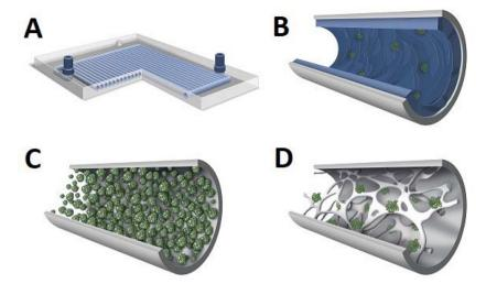
Fig. 1 Types of microreactors: lab-on-the-chip (A), capillary (B), packed-bed (C), and structural/monolithic (D)
