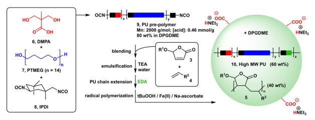
Fig. 2 Methodology for producing aqueous polyurethane/poly-butenolide hybrid dispersions.
