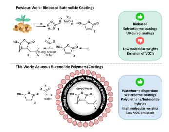
**Fig. 1** Previous work: biobased coating binder technology based on poly-butenolides using photo-oxidation, condensation, and co-polymerization.  $^{6,10-12}$  This work: waterborne polyurethane/poly-butenolide hybrid dispersions.
