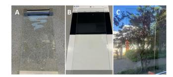
Fig. 4 Coating of PU/(3b + NVP) dispersion with a ratio of 40/60. (A) Application of dispersion on glass plate. (B) In front of black/white paper after application but before drying. (C) Clear, hard coating in front of window after drying.
