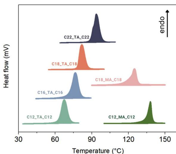
**Fig. 2** DSC traces showing the second heating cycle for the tartaric acid diesters (C<sub>12</sub>\_TA\_C<sub>12</sub>, C<sub>16</sub>\_TA\_C<sub>16</sub>, C<sub>18</sub>\_TA\_C<sub>18</sub>, and C<sub>22</sub>\_TA\_C<sub>22</sub>) and the first heating cycle of the mucic acid diesters (C<sub>12</sub>\_MA\_C<sub>12</sub> and C<sub>18</sub>\_MA\_C<sub>18</sub>), at a ramp rate of 10 °C min<sup>-1</sup>.
