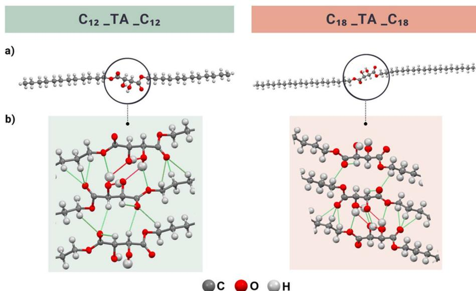
**Fig. 5** (a) Lattice structure of  $C_{12\_TA\_C_{12}}$  and  $C_{18\_TA\_C_{18}}$  and (b) hydrogen bonding and core group interactions (red represents strong hydrogen bonds and green represents non-classical hydrogen bonds) in  $C_{12\_TA\_C_{12}}$  and  $C_{18\_TA\_C_{18}}$ , viewed down the  $b$  axis.
