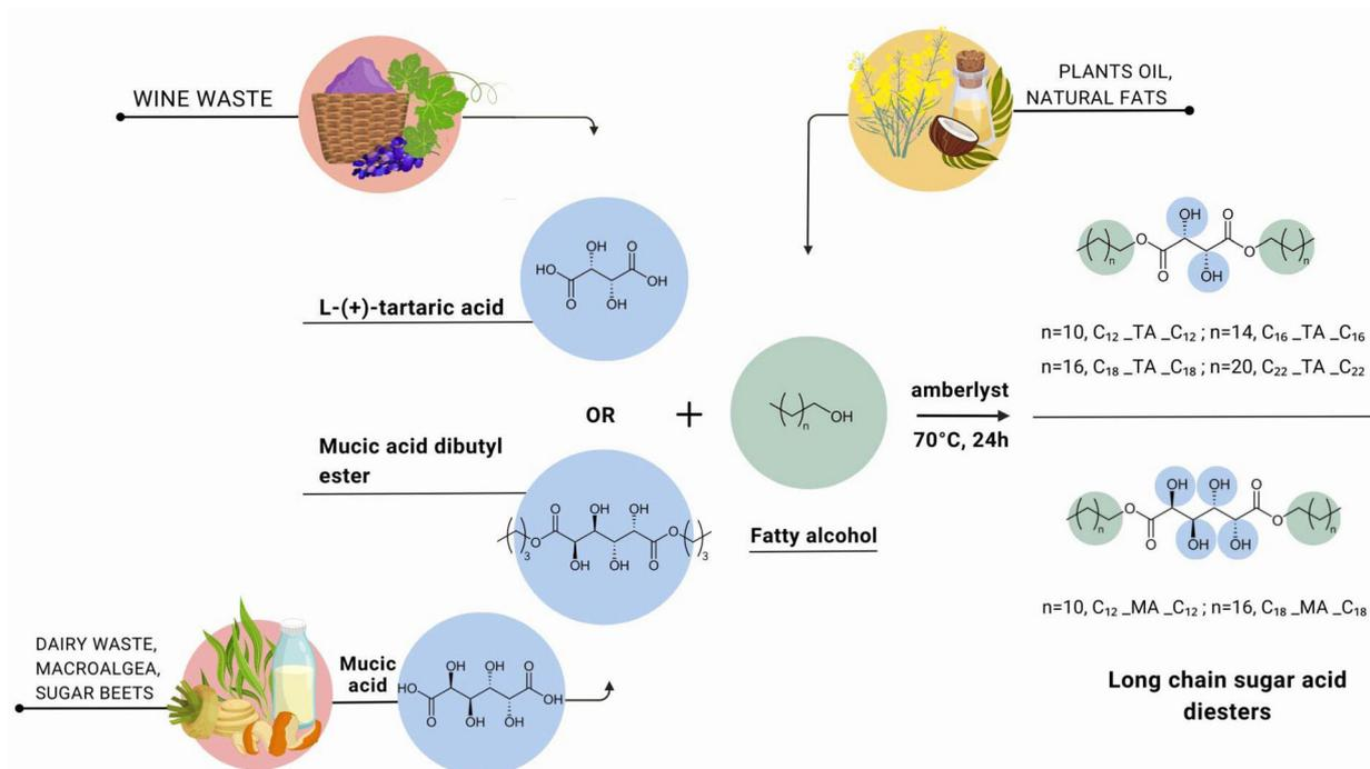
**Fig. 1** Scheme of synthesis of long-chain tartaric acid diesters ( $C_{12\_TA\_C_{12}}$ ,  $C_{16\_TA\_C_{16}}$ ,  $C_{18\_TA\_C_{18}}$ , and  $C_{22\_TA\_C_{22}}$ ) and mucic acid diesters ( $C_{12\_MA\_C_{12}}$  and  $C_{18\_MA\_C_{18}}$ ).
