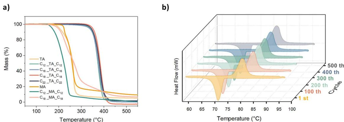
**Fig. 3** (a) TGA curves of tartaric acid ( $C_{12\_TA\_C_{12}}$ ,  $C_{16\_TA\_C_{16}}$ ,  $C_{18\_TA\_C_{18}}$ , and  $C_{22\_TA\_C_{22}}$ ), mucic acid diester ( $C_{12\_MA\_C_{12}}$  and  $C_{18\_MA\_C_{18}}$ ) and their precursors (TA and MA) at a  $10\text{ }^{\circ}\text{C min}^{-1}$  heating rate, and (b) latent heat values of  $C_{18\_TA\_C_{18}}$  after different thermal cycles, at a ramp rate of  $10\text{ }^{\circ}\text{C min}^{-1}$ .
