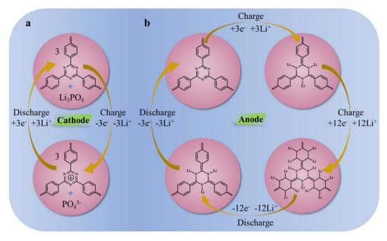
Fig. 5 Charge storage mechanism during the charging and discharging of (a) the cathode and (b) the anode.
