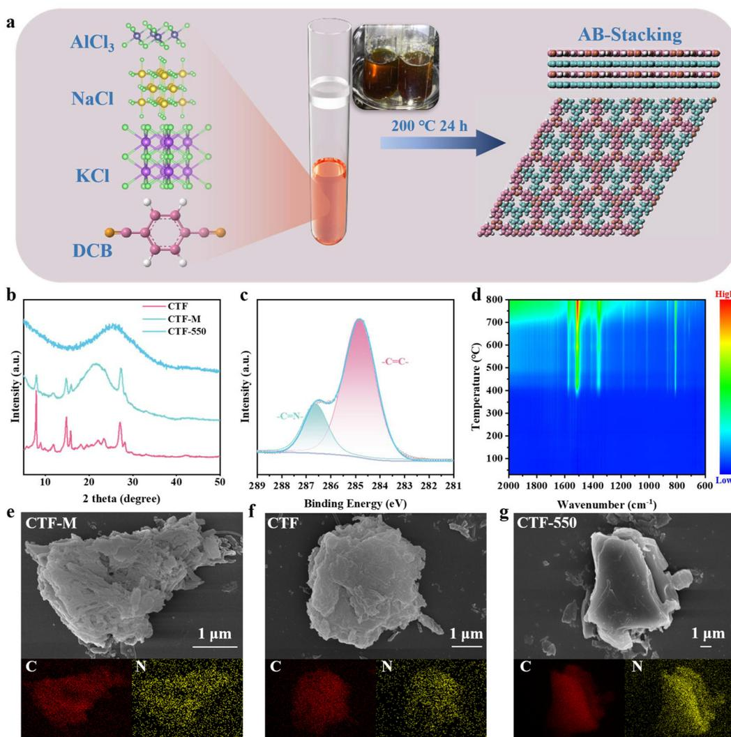
**Fig. 1** (a) Illustration of the preparation process of CTFs. (b) The XRD patterns of CTF, CTF-M and CTF-550. (c) The C 1s XPS spectra of CTF. (d) The TG-FTIR spectra of CTF. The SEM images and C and N elemental mapping images of (e) CTF-M, (f) CTF, (g) CTF-550.
