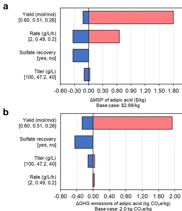
**Fig. 8** Single-point sensitivity analysis of parameters related to MA fermentation over the (a) MSP and (b) GHG emissions of producing AA from DMR sugars. Baseline fermentation parameters to generate the MSP of \$2.88 per kg of AA and the GHG emissions of 2.0 kg CO<sub>2</sub>e per kg AA are presented in parentheses, while extreme range points are indicated below each label. All data shown in this figure are provided in full in ESI 1.†
