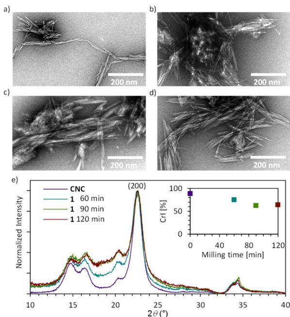
**Fig. 2** TEM images of (a) HCl hydrolyzed CNCs as well as tosylated CNCs after (b) 60 min, (c) 90 min and (d) 120 min of ball milling. (e) XRD diffractograms of normalized samples of CNC, **1** 60 min, **1** 90 min and **1** 120 min. Inset shows a plot of the crystallinity index (CrI) versus milling time. For full TEM images see Fig. S7a–d.†
