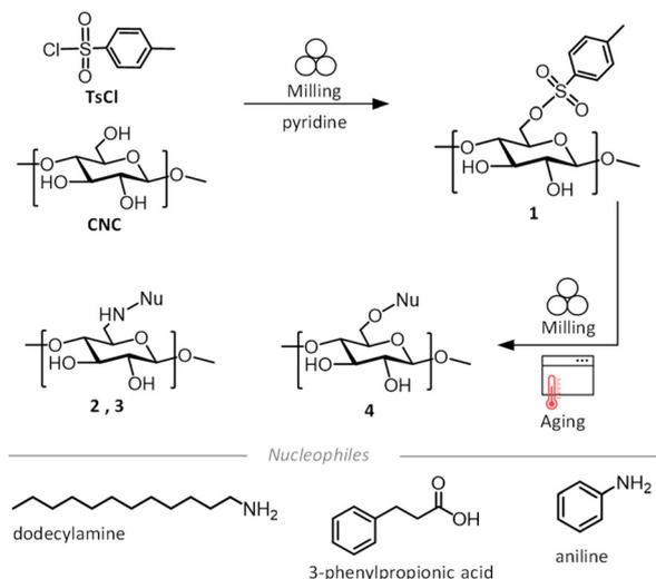
**Scheme 1** Reaction scheme of mechanochemically modified CNCs via implementing a tosylate as a leaving group and using the reactive intermediate (**1**) for attaching different functional groups, including dodecylamine, aniline and 3-phenylpropionic acid through solvent free nucleophilic substitution and form **2**, **3**, and **4** respectively.
