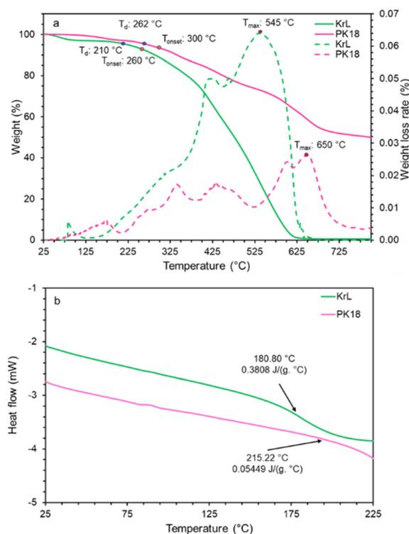
Fig. 9 Thermal analysis of KL and PK17. TGA curves with an arrow indicating *T<sub>max</sub>* (a). DSC curves showing the *T<sub>g</sub>* and *C<sub>p</sub>* (b).
