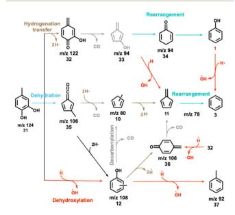
Scheme 7 CFP mechanism of 4-methylcatechol.
