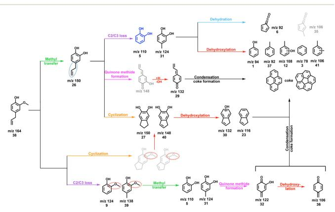
Scheme 8 The main initial decomposition pathways of eugenol in HZSM-5-catalyzed pyrolysis
