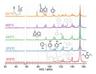
Fig. 2 Catalytic pyrolysis of syringol. Temperature-dependent mass spectra recorded at  $h\nu = 10.5$  eV upon syringol catalytic pyrolysis. Grey refers to potential products that could not be unambiguously identified. Reaction conditions: <0.1% syringol (m/z 154); H-ZSM-5 (Si/Al = 25); <0.5 bar; 20 sccm Ar.
