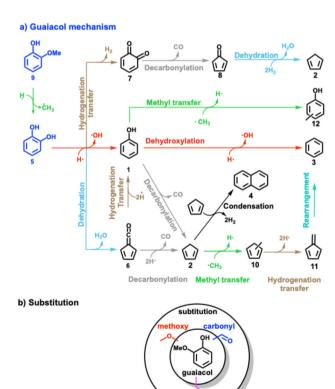
Scheme 2 (a) Overview of the reaction mechanism of the catalytic fast pyrolysis of guaiacol, catechol, phenol over H-ZSM-5 catalyst. The colour code for each reaction (dehydroxylation, methyl transfer, etc.) is consistent throughout the manuscript. (b) Overview of three substituted guaiacols investigated in this study.
