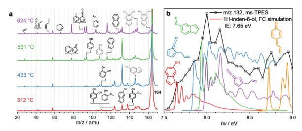
Fig. 3 (a) ToF MS recorded at  $h\nu = 10.5$  eV upon eugenol catalytic pyrolysis using HZSM-5. Grey structures denote potential or inconclusive assignments. Reaction conditions: <0.5% eugenol (m/z 164); HZSM-5 (Si/Al = 25); <0.5 bar; 20 sccm Ar. (b) The ms-TPES of m/z 132 evidences the formation of indenols and the quinone methide derivative, 4-allylidenecyclohexa-2,5-dien-1-one.
