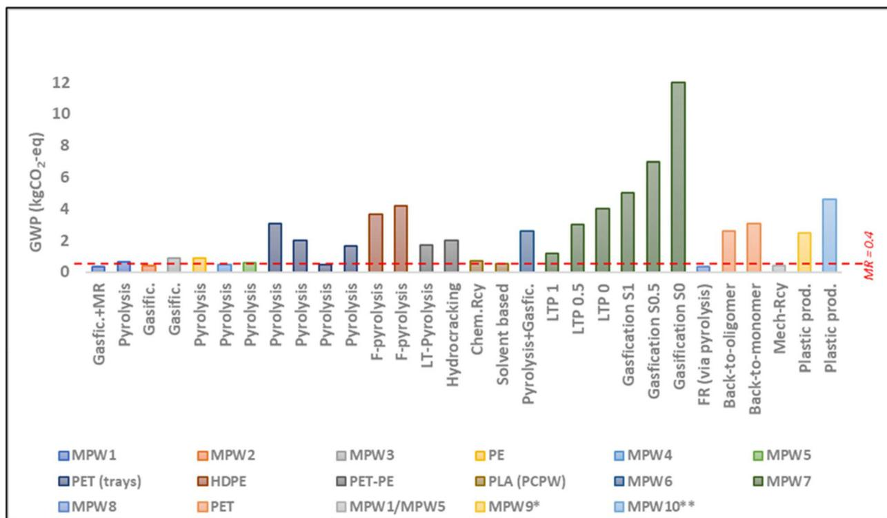
Fig. 9 GWP impact of plastic waste management *via* chemical recycling from 27 case studies (Gasific. = gasification; MR: mechanical recycling; F = fast; LTP = low-temperature pyrolysis; Rcy = recycling; FR = feedstock recycling), MPW = mixed plastic waste (see Table S1† for specific composition of each mix);\*cradle-to-gate plastic polymer production; \*\*cradle-to-grave (incineration of plastic waste).
