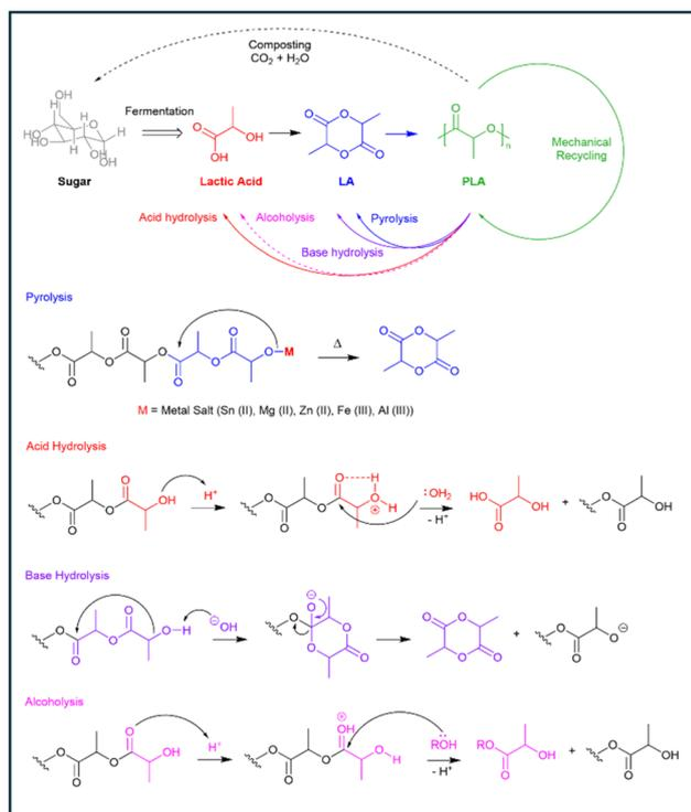
**Fig. 6** Illustration of different chemical recycling reactions for PLA and the corresponding products: pyrolysis (lactide); acid hydrolysis (lactic acid); base hydrolysis (lactide); and alcoholysis (alkyl lactate). Reproduced from ref. 155 with permission from MDPI, copyright 2020.
