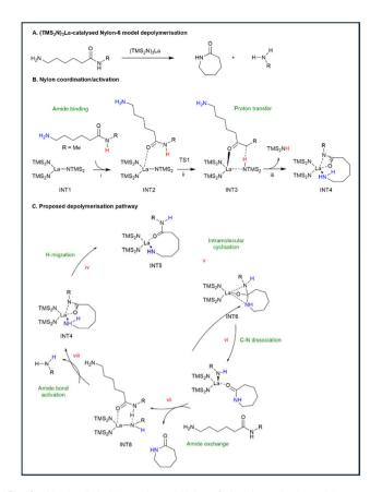
Fig. 8 Mechanistic illustration of Nylon-6 depolymerisation with commercially available lanthanide trisamido catalysts  $Ln(N(TMS)_2)_3$  (Ln = lanthanide). (A) Computed Nylon-6 model reaction. (B) Nylon coordination. (C) Proposed depolymerisation mechanism. Reproduced from ref. 175 with permission from Wiley, copyright 2023.
