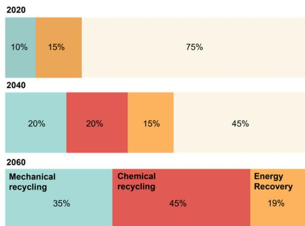
**Fig. 1** Plastic recycling outlook based on data from Nexant and Technip Energies. The percentage of plastics fall out of mechanical recycling, chemical recycling and energy recovery representing the stream that is sent for landfill (with leakage to nature). Reproduced from ref. 14 with permission from Holland Circular Hotspot, copyright 2023.
