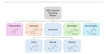
Fig. 2 Common PET chemical recycling routes and the associated main products.
