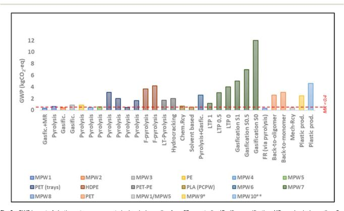
Fig. 9 GWP impact of plastic waste management via chemical recycling from 27 case studies (Gasific. = gasification; MR: mechanical recycling; F = fast; LTP = low-temperature pyrolysis; Rcy = recycling; FR = feedstock recycling), MPW = mixed plastic waste (see Table S1† for specific composition of each mix);\*cradle-to-gate plastic polymer production; \*\*cradle-to-grave (incineration of plastic waste).
