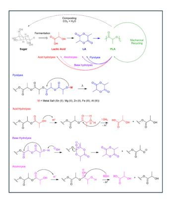
**Fig. 6** Illustration of different chemical recycling reactions for PLA and the corresponding products: pyrolysis (lactide); acid hydrolysis (lactide); base hydrolysis (lactide); and alcoholysis (alkyl lactate). Reproduced from ref. 155 with permission from MDPI, copyright 2020.
