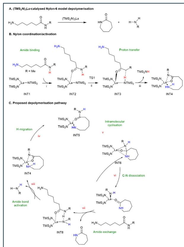
**Fig. 8** Mechanistic illustration of Nylon-6 depolymerisation with commercially available lanthanide trisamide catalysts  $\text{Ln}(\text{N}(\text{TMS})_2)_3$  (Ln = lanthanide). (A) Computed Nylon-6 model reaction. (B) Nylon coordination. (C) Proposed depolymerisation mechanism. Reproduced from ref. 175 with permission from Wiley, copyright 2023.
