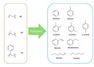
Fig. 3 Common products from polyolefin pyrolysis.
