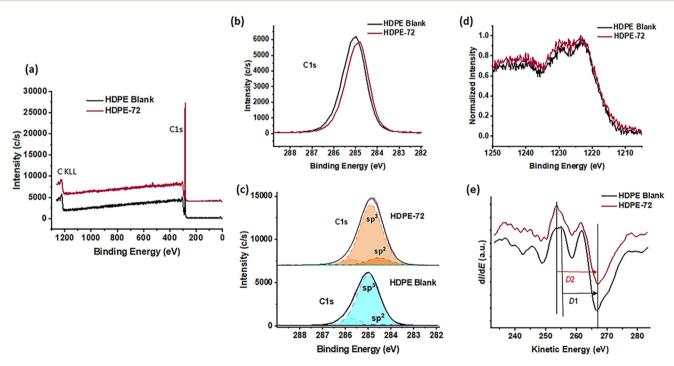
Fig. 4 Comparison of the XPS spectra of the blank HDPE and HDPE-72. In (a), (c) and (e), the two spectra are offset in the y-direction for better visualization. (a) Survey scans; (b) high-resolution scans for C 1s and (c) curve fitting of the envelope into composite peaks of sp<sup>2</sup>, sp<sup>3</sup> and vibrational fine structure (dashed lines); (d) X-ray excited carbon KLL Auger spectra; (e) first derivative of the carbon KLL Auger spectra obtained by numerical
