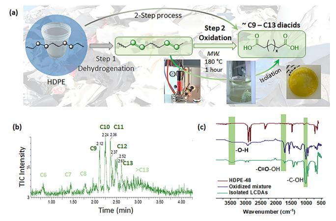
Fig. 5 (a) The microwave-assisted oxidation step of dehydrogenated HDPE to LCDA products using nitric acid as the oxidation reagent in a microwave reactor (Shelton, CT) for 1 hour at 180 °C under an  $N_2$  atmosphere; (b) UPLC-MS chromatograms of the oxidized fragments detected in the TIC channel, under the ESI-method; and (c) the FTIR spectra comparison of the dehydrogenated HDPE and the oxidative products.
