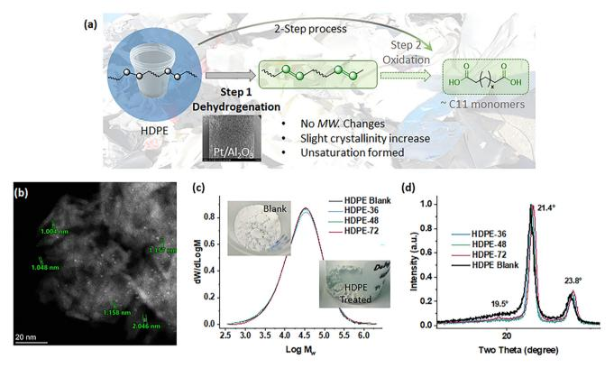
Fig. 2 Upcycling of HDPE via a two-step process: (a) schematic flow with the first dehydrogenation step using 1 wt% Pt/Al<sub>2</sub>O<sub>3</sub> in dry toluene and treated for 36-72 hours at 250 °C under N2; (b) STEM micrograph of the catalyst (Pt/Al2O3) used; (c) GPC traces of the HDPEs with images before and after treatment; and (d) XRD patterns of HDPEs with enlarged area of the spectra between 16° and 26°.
