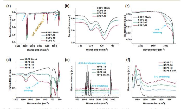
Fig. 3 (a) FTIR spectra of the HDPE before (blank) and after dehydrogenation (HDPE-36, 48, 72), with (b) enlarged area of the CH<sub>2</sub> stretching range, (c) the =CH- stretching range, (d) the =CH- bending geminal disubstituted alkene range, (e) Raman spectra of the HDPEs before and after dehydrogenation treatment, and (f) the enlarged area at the C=C stretching range.
