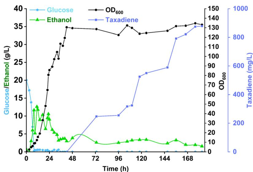
**Fig. 6** Fed-batch fermentation of the strain yZCL137 in a 5 L bioreactor. Fed-batch fermentations were performed at a 2.0 L scale using YPD medium and the engineered *S. cerevisiae* strain yZCL137.  $OD_{600}$  and glucose, ethanol, and taxadiene curves during fed-batch fermentation. Black arrows indicate the addition of *n*-dodecane and galactose to the medium. Error bars represent the means  $\pm$  SD from three biological replicates.
