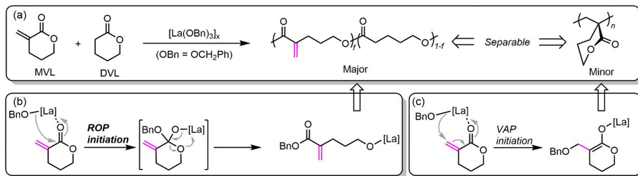
**Scheme 5** (a) General reaction scheme for the separable product mixture of  $P(MVL-co-VL)$  and  $P(MVL)_{VAP}$  from the polymerization of 30 wt% MVL in DVL with  $[La(OBn)_3]_x$ . (b) Competing initiation pathways: ring-opening of MVL or DVL with  $[La(OBn)_3]_x$  acting as a coordination insertion catalyst (left) and vinyl addition of MVL with  $[La(OBn)_3]_x$  acting as a coordination addition catalyst (right).
