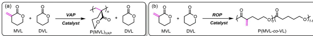
**Scheme 3** Proposed (co)polymerization strategies to separate the MVL/DVL mixture into (co)polymer and monomer products. (a) Vinyl-addition polymerization pathway to  $P(MVL)_{VAP}$  and DVL. (b) Ring-opening polymerization pathway to copolyester  $P(MVL-co-VL)$ .
