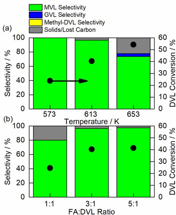
Fig. 2 Product distribution and DVL conversion over CaO/SiO<sub>2</sub> as a function of (a) reaction temperature (contact time of 0.27 h, 0.4 kPa DVL, 1.2 kPa FA, 0.1 g catalyst, 101 kPa) and (b) FA : DVL ratio (613 K, contact time of 0.27 h, 0.4 kPa DVL, 100 mg catalyst, 101 kPa).
