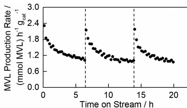
Fig. 3 MVL production rate (per g<sub>cat</sub>) as a function of time on stream (613 K, contact time of 0.27 h, 0.4 kPa DVL, 1.2 kPa FA, 101 kPa). Dashed lines represent a regeneration in 50 mL min<sup>-1</sup> of air for 4 h.
