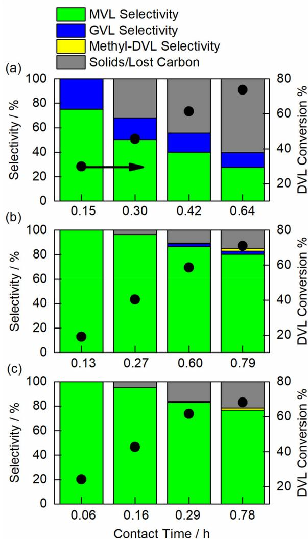
Fig. 1 Product distributions and DVL conversions as functions of contact time for (a) MgO/SiO<sub>2</sub>, (b) CaO/SiO<sub>2</sub> and (c) BaO/SiO<sub>2</sub> (613 K, 0.1 g catalyst, 0.4 kPa DVL, 1.2 kPa FA, 101 kPa, balance N<sub>2</sub>).
