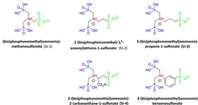
**Fig. 9** Schematic structures of phosphonate scale inhibitors subjected to seawater biodegradation over 28 days (BOD<sub>28</sub>) by the OECD 306 method.
