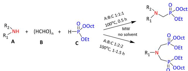
Scheme 11 MW-assisted synthesis of ethyl octyl  $\alpha$ -aminophosphonates.
