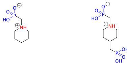
Fig. 25 Schematic structures of the corrosion inhibitors piperidin-1-yl-phosphonic acid (PPA) and (4-phosphono-piperidin-1-yl)phosphonic acid (PPPA).
