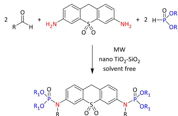
**Scheme 18** Silica-supported TiO<sub>2</sub>-catalyzed synthesis of bis(α-aminophosphonates).
