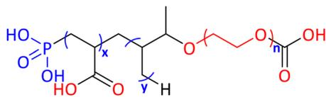
Fig. 16 Schematic structure of AA-APEM-H<sub>3</sub>PO<sub>3</sub> polymer as CaCO<sub>3</sub> scale inhibitor.
