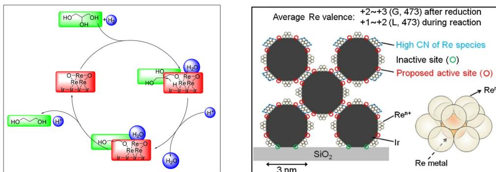
Fig. 17 Potential reaction pathway for glycerol hydrogenolysis over Ir-ReO<sub>x</sub>/SiO<sub>2</sub> (left) and model structure of Ir-ReO<sub>x</sub>/SiO<sub>2</sub> (20 wt%-Ir, Re/Ir = 0.34, actual) during the reaction (right).<sup>149,150</sup>
