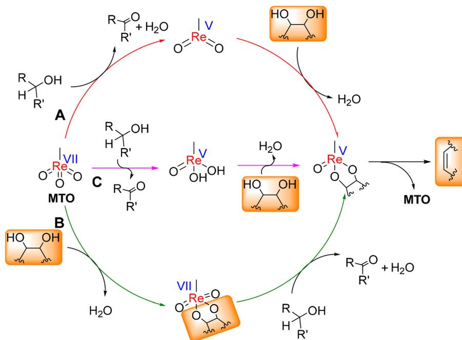
**Fig. 5** Proposed mechanism C and alternative mechanisms A and B for deoxydehydration reaction of diols over MTO catalysts with alcohol reductants<sup>78</sup> (MTO: methyltrioxorhenium).
