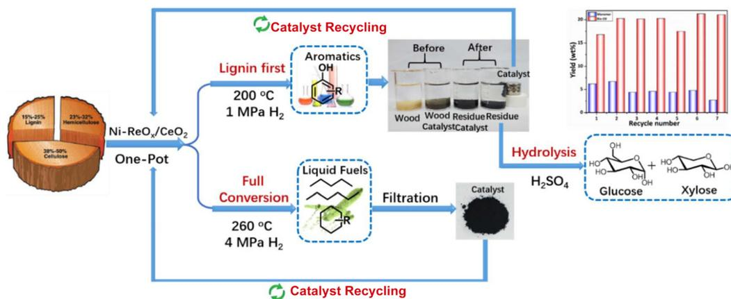
Fig. 13 Conversion of woody biomass to aromatics and alkanes over Ni–ReO<sub>x</sub>/CeO<sub>2</sub>.<sup>45</sup>
