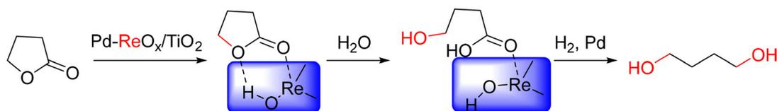
Fig. 16 Schematic reaction pathway for the conversion of  $\gamma$ -butyrolactone to 1,4-butanediol.<sup>133</sup>
