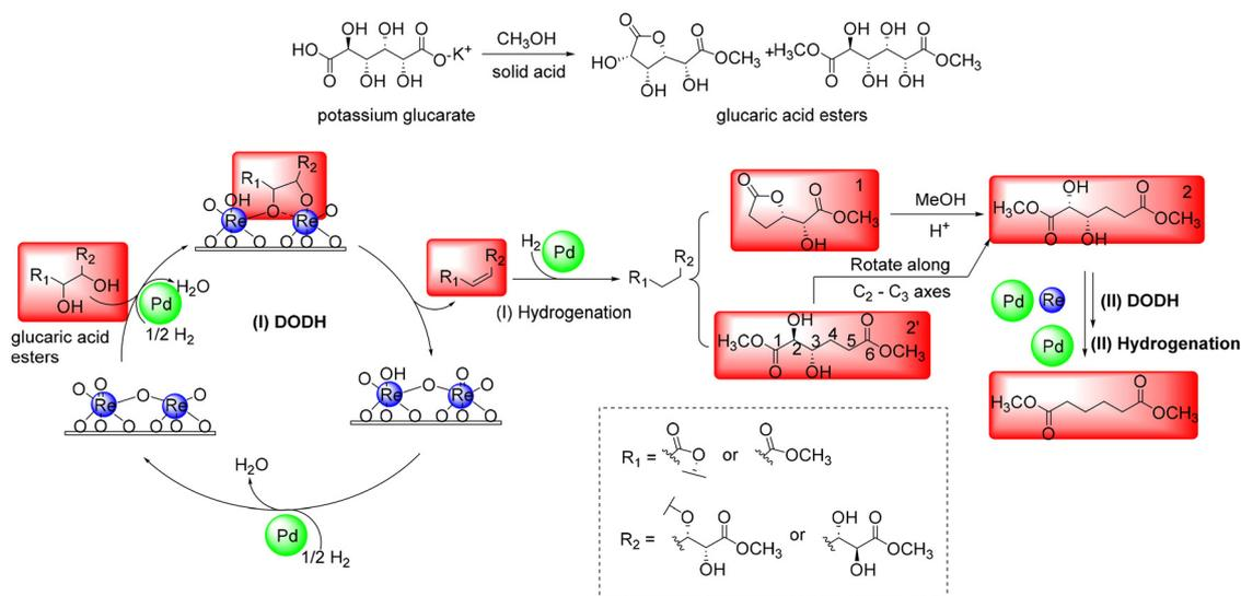
**Fig. 19** Proposed reaction mechanism for the conversion of gluconic acid (potassium gluconate) to adipic acid (methyl adipate) catalyzed by Pd- $\text{ReO}_x/\text{AC}^{175}$  (DODH: deoxydehydration).
