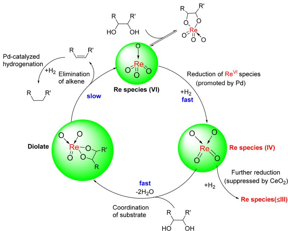
Fig. 18 Proposed reaction mechanism for the deoxydehydration reaction over  $\text{ReO}_x$  catalysts.<sup>162</sup>
