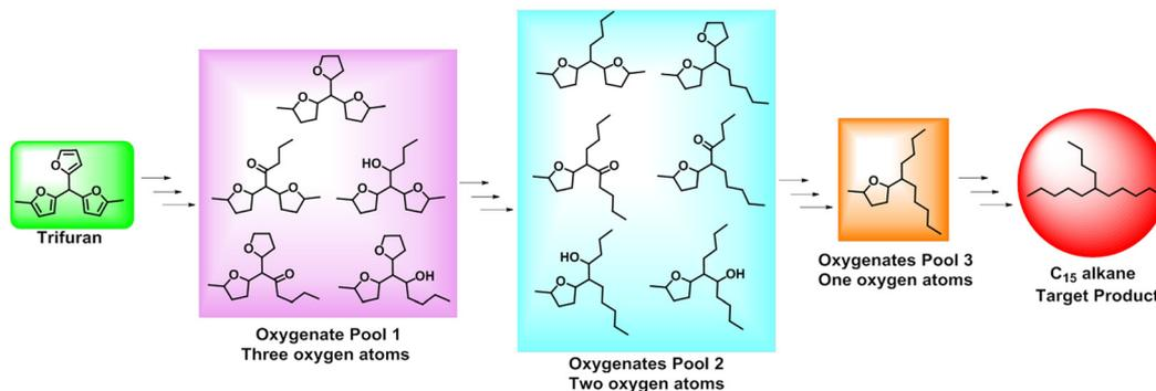
**Fig. 20** Intermediate oxygen-containing compounds generated during the trifuran conversion process over an Ir- $\text{ReO}_x/\text{SiO}_2$  catalyst were discerned *via* GC-MS analysis of the resultant product solutions.<sup>180</sup>
