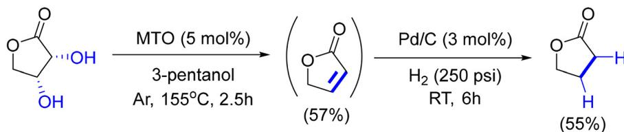
**Fig. 6** Conversion of *D*-erythrone lactone to  $\gamma$ -butyrolactone *via* deoxydehydration and hydrogenation reactions with methyltrioxorhenium as the catalyst<sup>74</sup> (MTO: methyltrioxorhenium).
