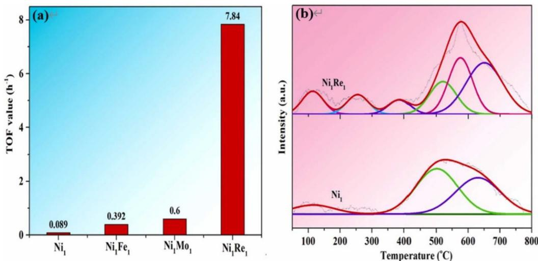
Fig. 15 (a) Comparison of TOF values over different reduced catalysts (0.1 g of fatty acid, 0.02 g of activated catalyst in 10 mL of cyclohexane solvent at 150 °C and 4.0 MPa hydrogen); (b) H<sub>2</sub>-TPD profiles of the reduced Ni<sub>1</sub> and Ni<sub>1</sub>Re<sub>1</sub> catalysts.<sup>124</sup>
