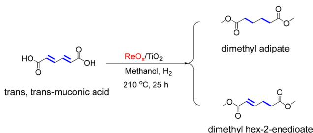
Fig. 14 Hydrogenation of muconic acid into different adipic acid esters in methanol over ReO<sub>x</sub>/TiO<sub>2</sub> catalysts.<sup>114</sup>
