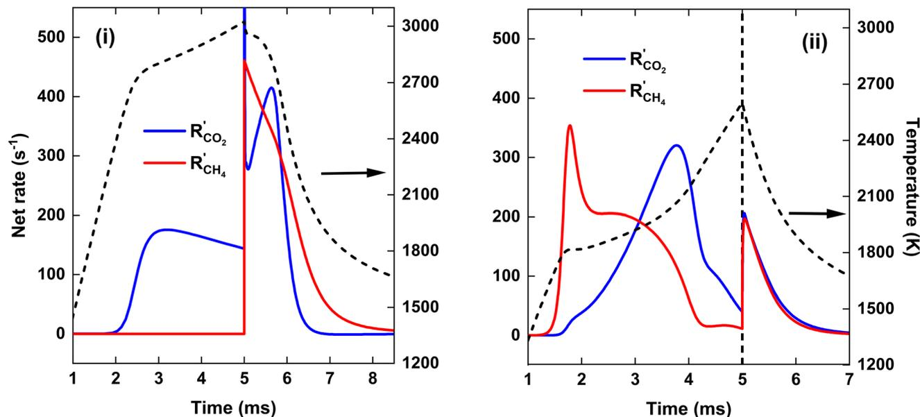
Fig. 8 Net rates of conversion of CO<sub>2</sub> and CH<sub>4</sub>, as a function of time, for SEI = 140 kJ mol<sup>-1</sup> (left y-axis). The temperature is indicated by the dashed black line (right y-axis). The left panel (i) and right panel (ii) show the results for the CO<sub>2</sub> plasma with post-plasma CH<sub>4</sub> injection, and for the CO<sub>2</sub>/CH<sub>4</sub> plasma with post-plasma CO<sub>2</sub>/CH<sub>4</sub> injection, respectively.
