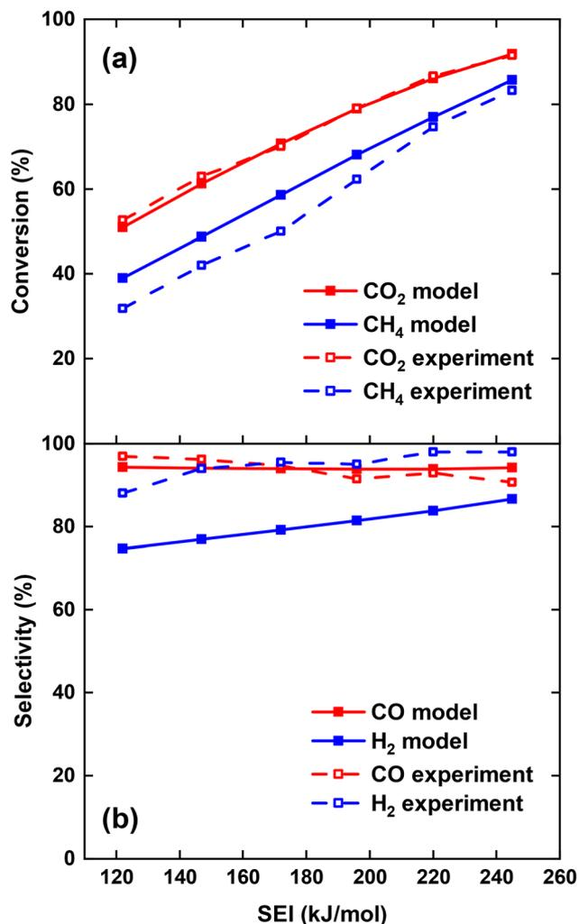
Fig. 1 Comparison of CO<sub>2</sub> and CH<sub>4</sub> conversion (a) and CO and H<sub>2</sub> selectivity (b) between model and experiment,<sup>17</sup> as a function of the SEI.
