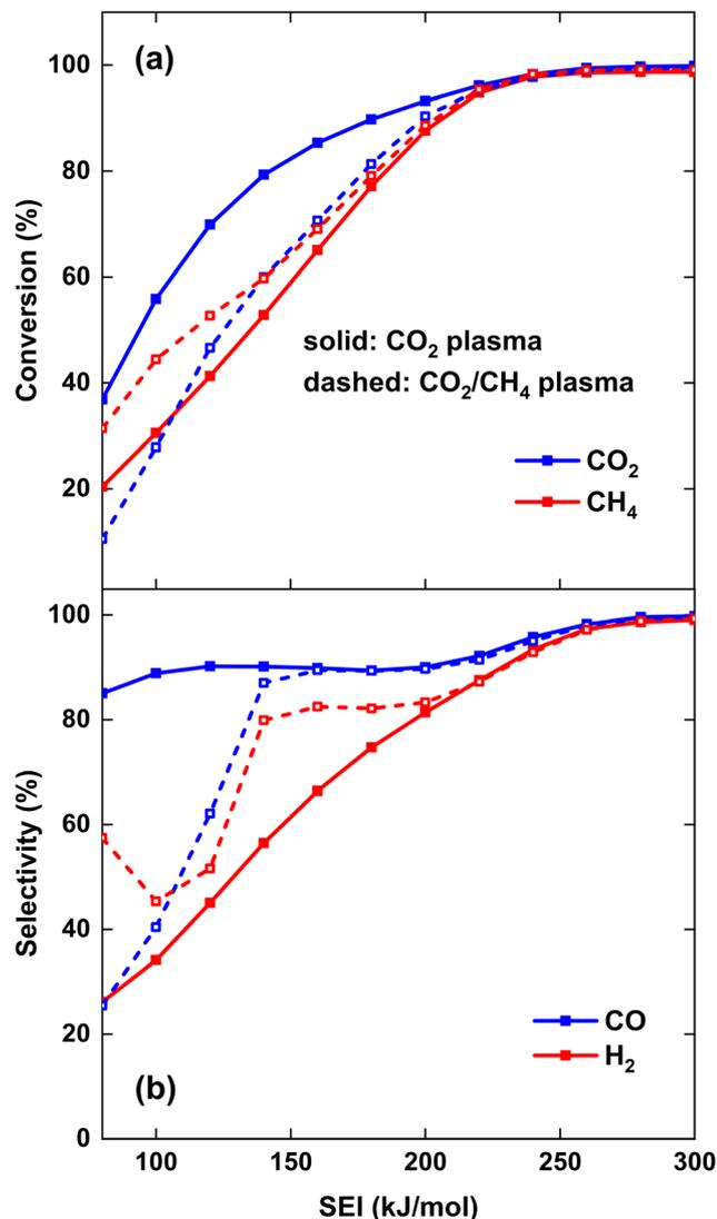
Fig. 5 CO<sub>2</sub> and CH<sub>4</sub> conversion (a) and CO and H<sub>2</sub> selectivity (b) as a function of the SEI. The solid and dashed lines indicate the results for the CO<sub>2</sub> plasma with post-plasma CH<sub>4</sub> injection, and for the CO<sub>2</sub>/CH<sub>4</sub> plasma with post-plasma CO<sub>2</sub>/CH<sub>4</sub> injection, respectively.
