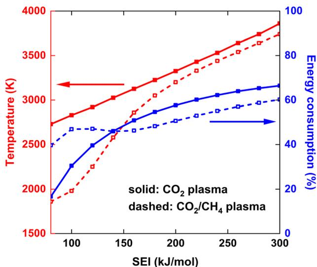
Fig. 4 Maximum gas temperature at the end of the plasma ( $t = 5$  ms) (left y-axis) and (fractional) energy consumption in the plasma (right y-axis), as a function of the SEI. The solid and dashed lines indicate the results for the  $\text{CO}_2$  plasma with post-plasma  $\text{CH}_4$  injection, and for half of the  $\text{CO}_2/\text{CH}_4$  mixture injected into the plasma and the other half of the  $\text{CO}_2/\text{CH}_4$  mixture injected post-plasma, respectively.
