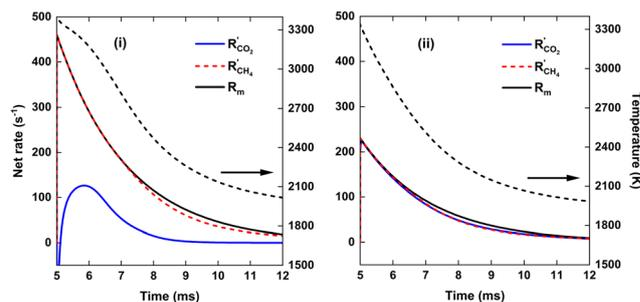
**Fig. 10** Net rates of conversion of CO<sub>2</sub> and CH<sub>4</sub> and mixing rate (solid black line) as a function of time, for SEI = 220 kJ mol<sup>-1</sup> (left y-axis). The temperature is indicated by the dashed black line (right y-axis). The left panel (i) and right panel (ii) show the results for the CO<sub>2</sub> plasma with post-plasma CH<sub>4</sub> injection, and for the CO<sub>2</sub>/CH<sub>4</sub> plasma with post-plasma CO<sub>2</sub>/CH<sub>4</sub> injection, respectively.
