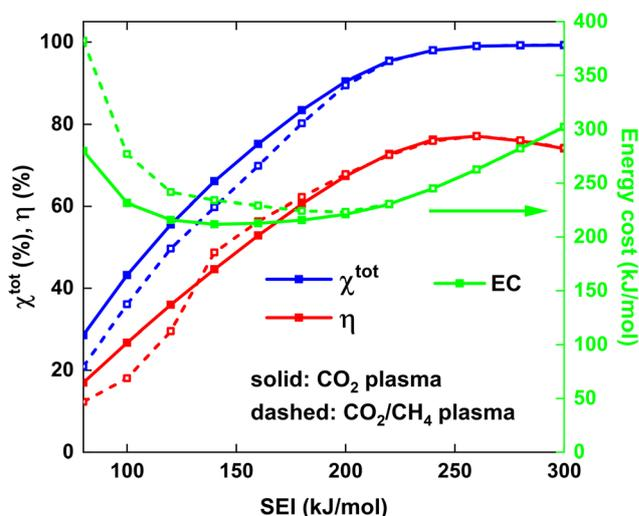
Fig. 6 Total conversion and ECE (left y-axis) and EC of conversion (right y-axis) as a function of the SEI. The solid and dashed lines indicate the results for the CO<sub>2</sub> plasma with post-plasma CH<sub>4</sub> injection, and for the CO<sub>2</sub>/CH<sub>4</sub> plasma with post-plasma CO<sub>2</sub>/CH<sub>4</sub> injection, respectively.
