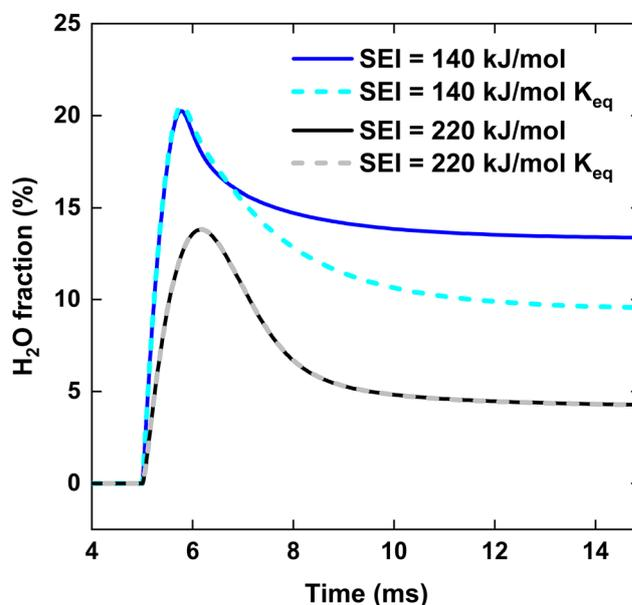
Fig. 12 H<sub>2</sub>O fraction as a function of time, for the CO<sub>2</sub> plasma with post-plasma CH<sub>4</sub> injection, at SEI = 140 kJ mol<sup>-1</sup> and SEI = 220 kJ mol<sup>-1</sup>. The dashed lines indicate the H<sub>2</sub>O fraction predicted by the WGS equilibrium.
