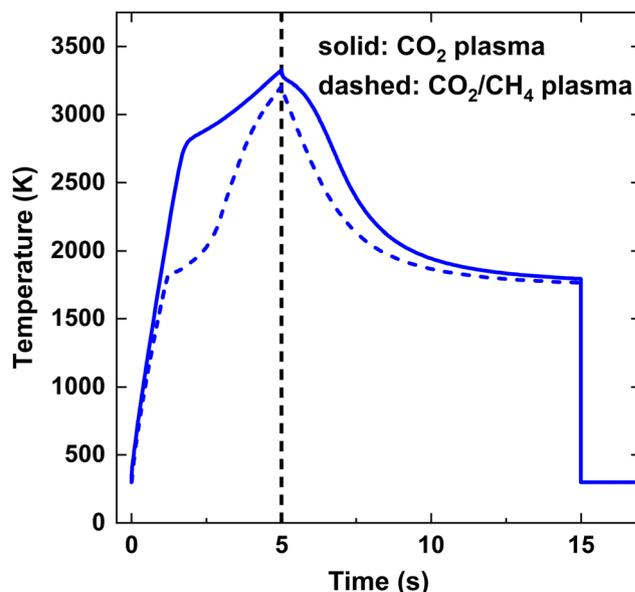
Fig. 3 Gas temperature as a function of time for SEI = 200 kJ mol<sup>-1</sup>. The black vertical dashed line at  $t = 5$  ms indicates the onset of post-plasma injection.
