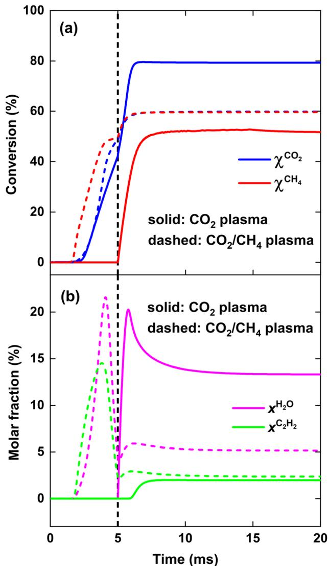
Fig. 7 CO<sub>2</sub> and CH<sub>4</sub> conversion (a), as well as H<sub>2</sub>O and C<sub>2</sub>H<sub>2</sub> molar fraction (b), as a function of time, for SEI = 140 kJ mol<sup>-1</sup>. The solid and dashed lines indicate the results for the CO<sub>2</sub> plasma with post-plasma CH<sub>4</sub> injection, and for the CO<sub>2</sub>/CH<sub>4</sub> plasma with post-plasma CO<sub>2</sub>/CH<sub>4</sub> injection, respectively. The vertical dashed line at 5 ms indicates the post-plasma mixing.
