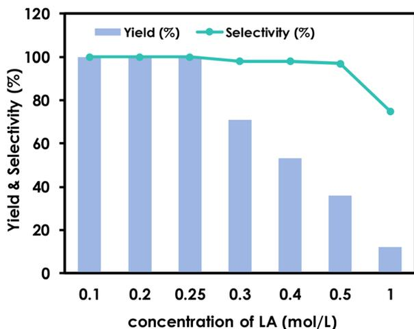
**Fig. 3** Effects of LA concentration for decarboxylative protonation of LA. Reaction conditions: 0.5 mmol LA, 0.05 mmol 9-mesityl-2,7-di-*tert*-butyl-10-acridine (A5) (10 mol%), 0.025 mmol 4-Cl-PhSH (5 mol%), *x* mL DCM (0.25 M), 400 nm LEDs (20 W), Ar, room temperature (RT), 20 h. Yield and selectivity were determined by GC with *n*-dodecane as the internal standard.
