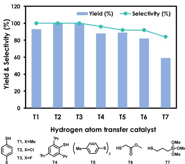
**Fig. 1** Effects of hydrogen atom transfer catalysts for decarboxylative protonation of LA. Reaction conditions: 0.5 mmol LA, 0.05 mmol 9-mesityl-2,7-di-*tert*-butyl-10-acridine (**A5**) (10 mol%), 0.025 mmol thiophenol or thiol (5 mol%), 2.0 mL DCM (0.25 M), 400 nm LEDs (20 W), Ar, room temperature (RT), 20 h. Yield and selectivity were determined by GC with *n*-dodecane as the internal standard.
