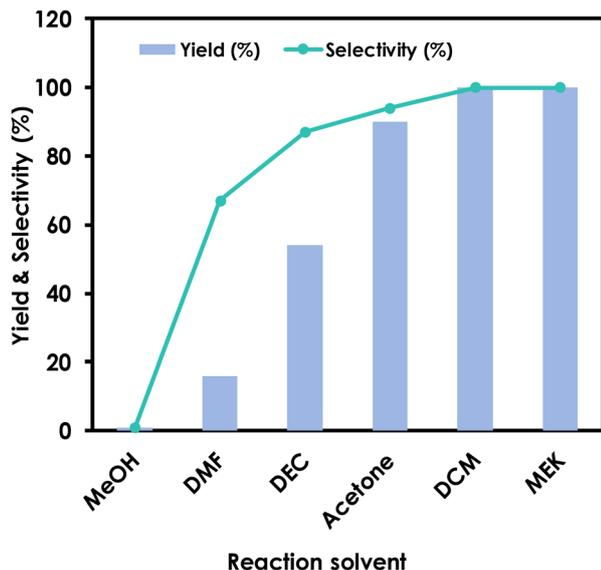
**Fig. 2** Effects of solvents for decarboxylative protonation of LA. Reaction conditions: 0.5 mmol LA, 0.05 mmol 9-mesityl-2,7-di-*tert*-butyl-10-acridine (A5) (10 mol%), 0.025 mmol 4-Cl-PhSH (5 mol%), 2.0 mL solvent (0.25 M), 400 nm LEDs (20 W), Ar, room temperature (RT), 20 h. Yield and selectivity were determined by GC with *n*-dodecane as the internal standard.
