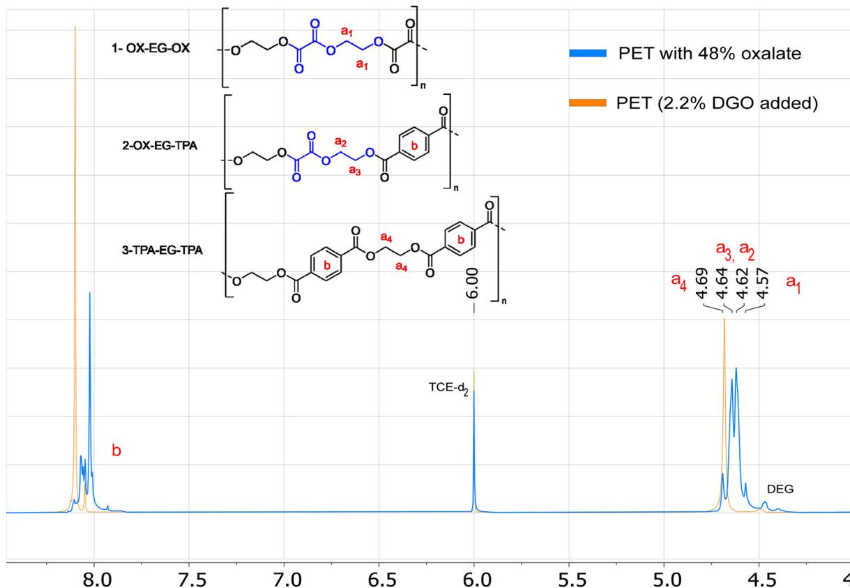
**Fig. 6** Superimposed  $^1\text{H}$  NMR spectra of the molecular weight boosted PET (2.2 mol%) and PETO with 48% oxalate. The blue spectrum represents the NMR spectrum of PETO with 48% oxalate and the orange spectra that of the PET produced by assistance of 2.2 mol% DGO. The chemical shifts of the different ethylene glycol oxalate and terephthalate esters are highlighted. The mentioned percentages are based on the total of diacids (terephthalate + oxalate).
