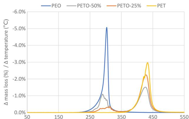
**Fig. 2** Oxalate removal upon heating (TGA). PET, polyethylene oxalate (PEO) and PET-oxalate copolymers (PETO) were subjected to heating at 10 °C min<sup>-1</sup>. The derivative of mass loss (%) with respect to temperature is given. The mentioned percentages of PETO represent the amount of oxalate in the polymer, expressed as fraction of the total acid (oxalate + terephthalate).
