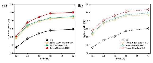
Fig. 1 Substrate hydrolyzability from surfactant-assisted glycerol organosolv pretreatment. (a) Glucose yield and (b) xylose yield.
