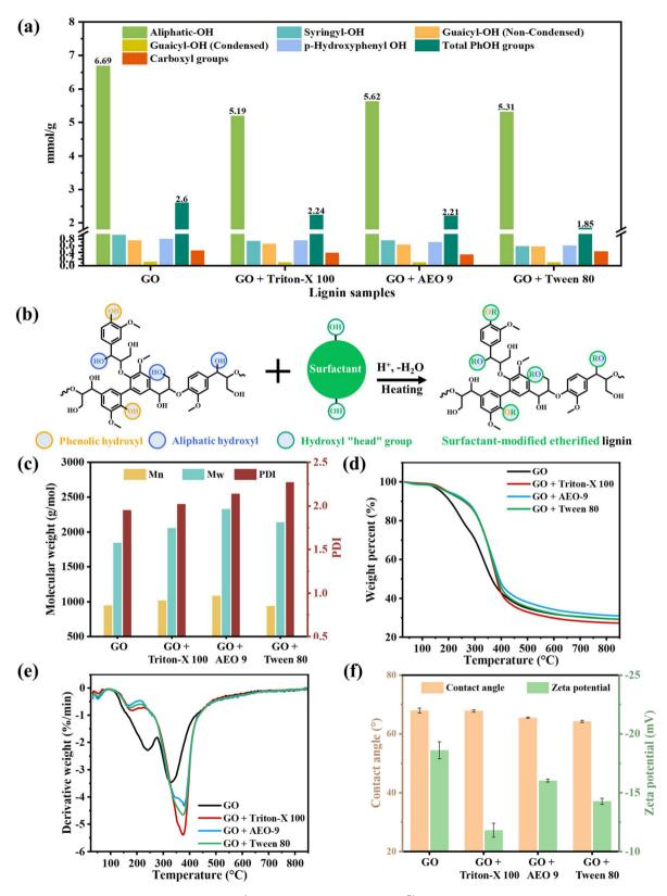
Fig. 3 (a) Quantification of functional groups (mmol  $g^{-1}$ ) in the residual lignin based on <sup>31</sup>P NMR; (b) proposed routes of surfactant modification on the lignin structure via etherification; (c) molecular weight distribution; (d) TG and (e) DTG curves of different lignin samples; and (f) contact angle measurement and zeta potential analysis.
