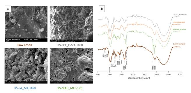
Fig. 6 (a) SEM photographs of the raw lichen and residual solids after SA-MAH160, SCF-MAH160 and MAH\_ML5-170 and (b) their FT-IR spectra.
