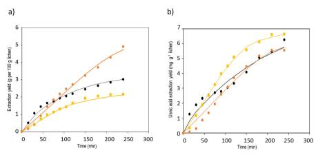
Fig. 1 Influence of the microwave (, 1 min 480 W; , 1 min 800 W) pretreatment on the supercritical carbon dioxide extraction from *Evernia pru-nastri* at 35 MPa and 40 °C and with 5% ethanol as cosolvent. (a) Overall extraction yield and (b) usnic acid extraction yield. Control experiment (). Lines represent Sovová's model fittings.
