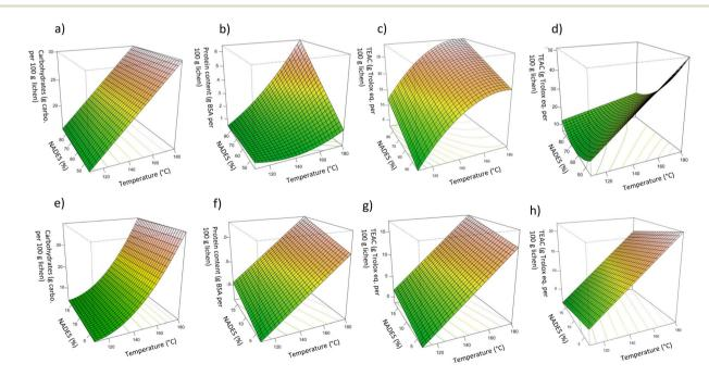
Fig. 3 Response surface for the effects of NaDES percentage and temperature in a range of high values with LA: Gly: W on (a) the extraction yield of carbohydrates, (b) the extraction yield of protein, (c) the ABTS antiradical capacity, and (d) for Men: Lau on the ABTS antiradical capacity, and in a range of low values with LA: Gly: W on (e) the extraction yield of carbohydrates, (f) the extraction yield of protein, and (g) TEAC, and (h) for Men: Lau on TEAC.
