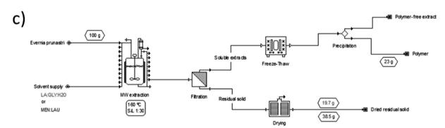
Fig. 5 Flow diagram of the different processes tested for the extraction of bioactives and biopolymers from *E. prunastri*: (a) SA-MAH160, (b) SFE\_E-MAH160 and (c) NADES-modified hydrothermal extraction with LA: Gly: W 80% at 170 °C (bioactives) or with Men: Lau 5% at 170 °C (polysaccharides).
