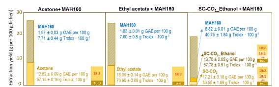
Fig. 2 Comparative performance of the three sequential processes: conventional Soxhlet acetone and ethyl acetate extraction and supercritical CO<sub>2</sub> extraction followed by microwave assisted hydrolysis at 160 °C (MAH160) regarding the total phenolic content, Trolox equivalent antioxidant capacity and fatty acid content from *Evernia prunastri*.
