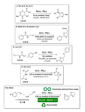
Fig. 1 Known approaches to the electrosynthesis of 2-oxazolines.
