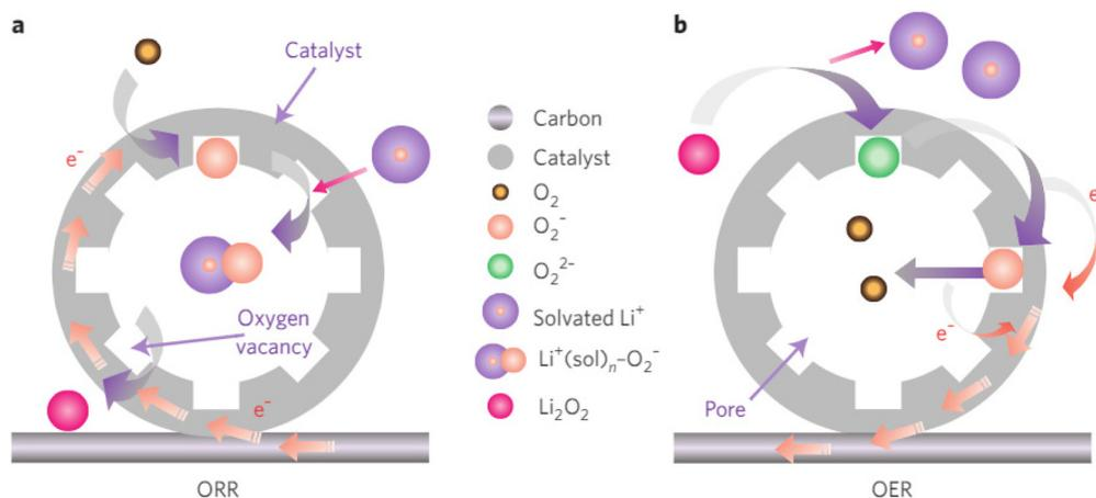
**Fig. 6** The mechanism of a porous oxygen-deficient oxide catalyst for Li–air batteries<sup>8</sup> (a) discharging (ORR) and (b) charging (OER).
