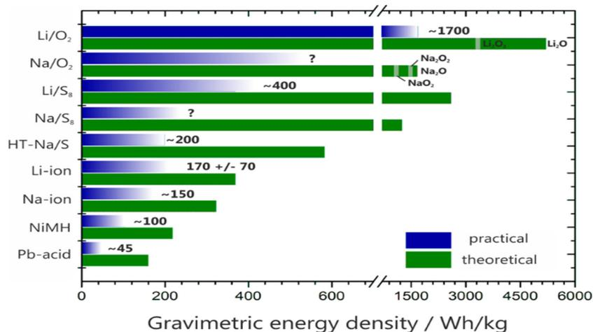
Fig. 2 The performance examination of theoretical and practical energy densities of several rechargeable batteries.<sup>72</sup>
