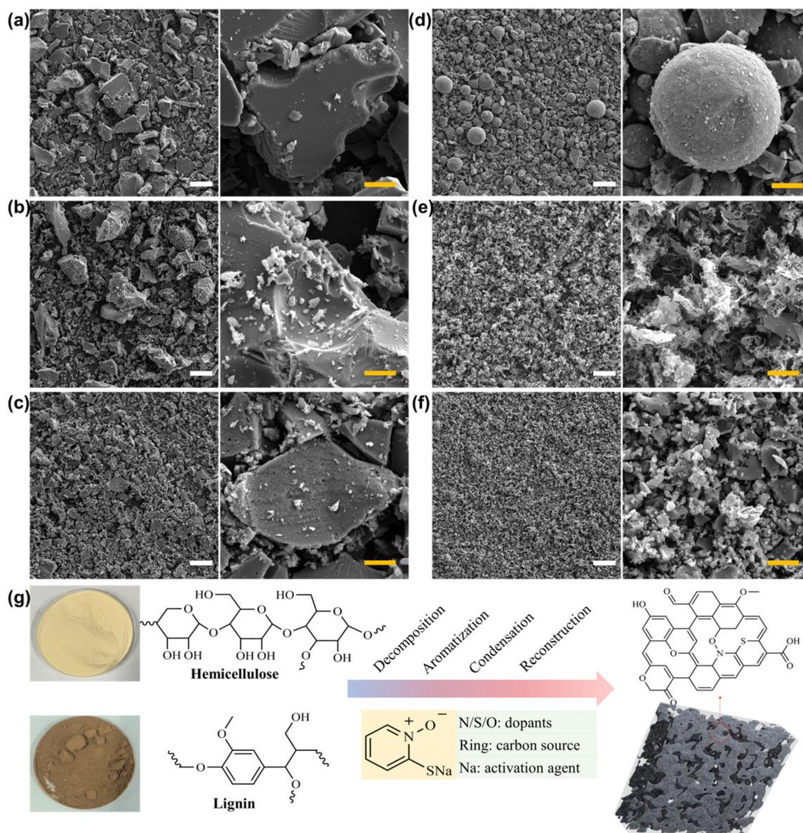
**Fig. 1** SEM images of lignin and hemicellulose-derived carbon materials at different magnifications: (a) LC, (b) SHLC, (c) SPLC, (d) HC, (e) SHHC, and (f) SPHC, (white bar: 50  $\mu\text{m}$ , yellow bar: 10  $\mu\text{m}$ ). (g) Schematic of the possible SP-derived carbon formation pathway.
