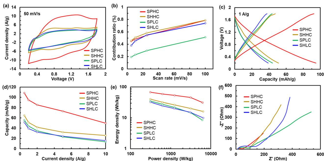
Fig. 3 Electrochemical analysis of ACs: (a) CV curves at 50  $mV s^{-1}$ , (b) capacitive contribution in cathodes at different scan rates, (c) CD profiles at 1  $A g^{-1}$ , (d) rate performance at different current densities, (e) Ragone plots, and (f) Nyquist plots.
