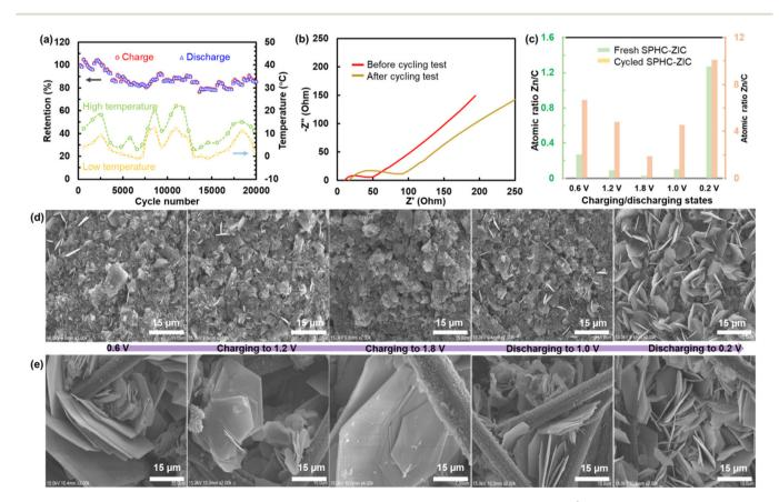
Fig. 4 (a) Cycling measurement performed on a SPHC cathode-based ZIC at ambient condition at 7 A g<sup>-1</sup>. (b) EIS profiles before and after the cycling test. (c) Atomic ratio of Zn/C at different voltages during the charging process. Images of the (d) fresh SPHC cathode and (e) cycled SPHC cathode at different states.
