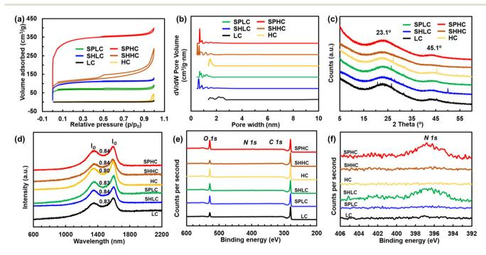
Fig. 2 (a) Nitrogen isotherms, (b) pore distributions, (c) XRD patterns, (d) Raman spectra, (e) XPS survey curves, and (f) high-resolution N 1s spectra of the produced carbons.
