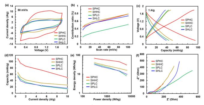
Fig. 3 Electrochemical analysis of ACs: (a) CV curves at 50 mV s<sup>-1</sup>, (b) capacitive contribution in cathodes at different scan rates, (c) CD profiles at 1 A g<sup>-1</sup>, (d) rate performance at different current densities, (e) Ragone plots, and (f) Nyquist plots.
