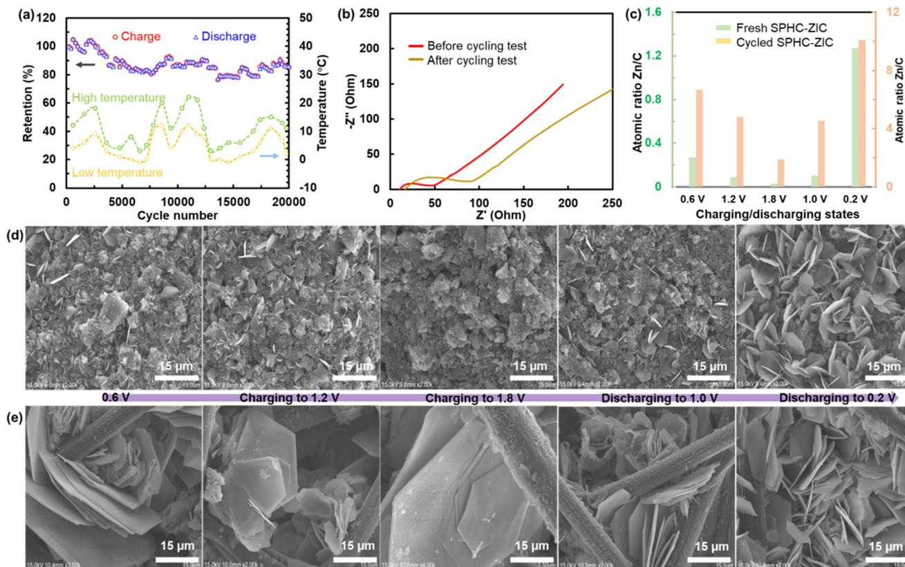
Fig. 4 (a) Cycling measurement performed on a SPHC cathode-based ZIC at ambient condition at  $7 \text{ A g}^{-1}$ . (b) EIS profiles before and after the cycling test. (c) Atomic ratio of Zn/C at different voltages during the charging process. Images of the (d) fresh SPHC cathode and (e) cycled SPHC cathode at different states.
