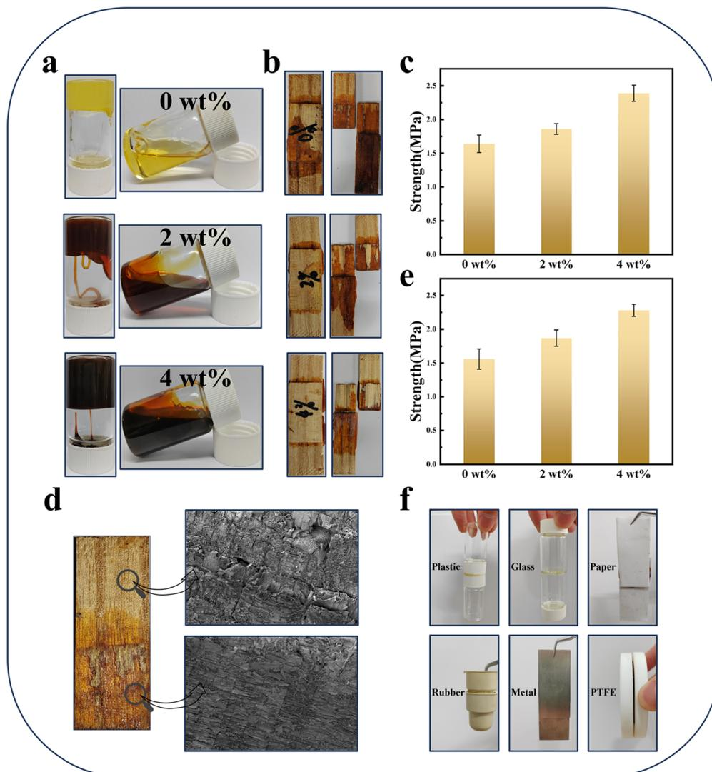
**Fig. 3** Photographs of the cellulose solutions with different concentrations at room temperature (left) and 100 °C (right) (a), the photographs of the adhesion of cellulose solutions to wood panels (b), the tensile strength of wood panels by cellulose solutions (c), the SEM photographs of the surface of the wood panel (d), the tensile strength of bamboo panels by cellulose solutions (e), and photographs of the adhesion of cellulose solutions to different substrates (f).
