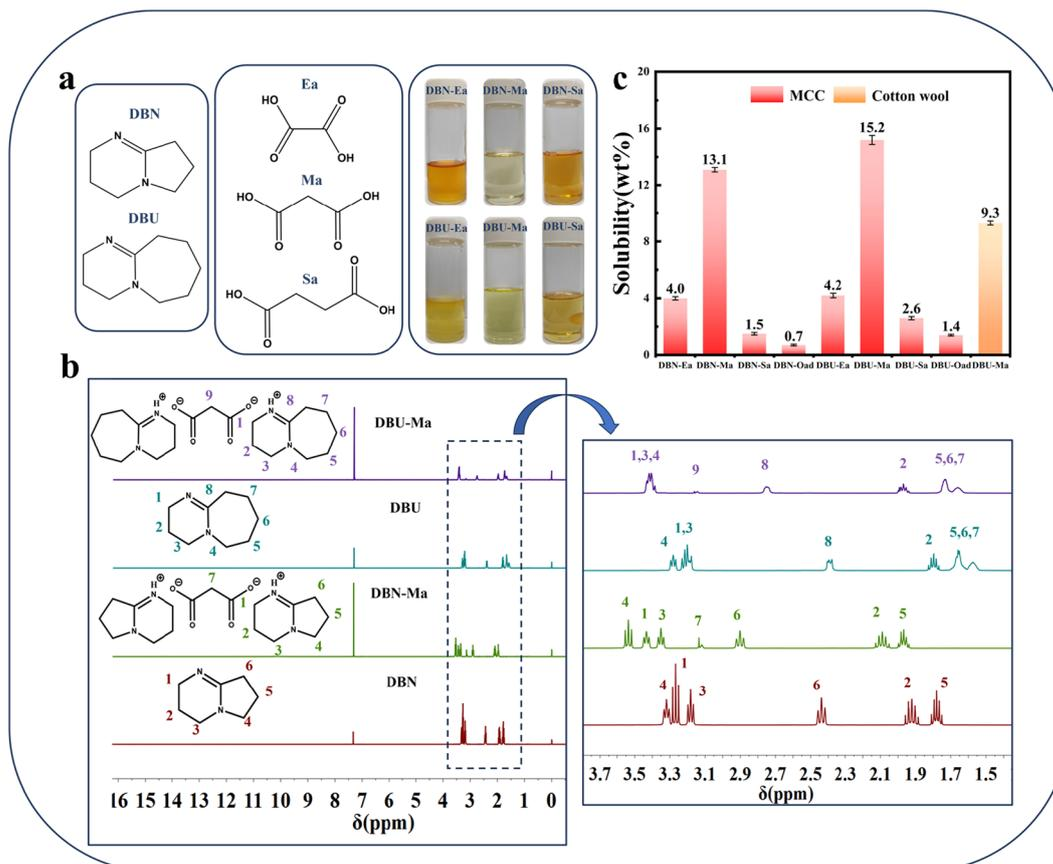
**Fig. 1** The composition and photographs of SILs (a), <sup>1</sup>H NMR spectra of DBN-Ma and DBU-Ma (b), and the solubility of cellulose by different SILs (c).
