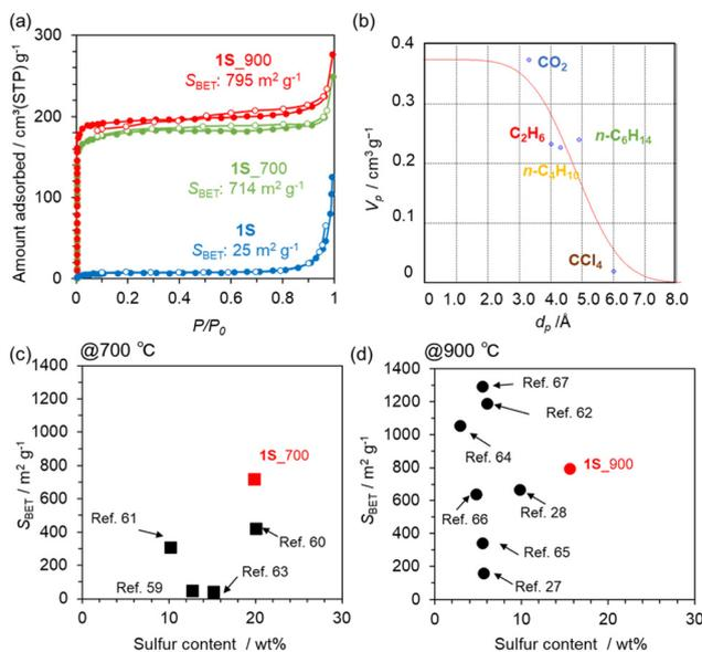
Fig. 4 (a) N<sub>2</sub> adsorption/desorption isotherms of **1S**, **1S**<sub>700</sub>, and **1S**<sub>900</sub> samples. (b) Micropore volume (*V*<sub>p</sub>) of **1S**<sub>900</sub> estimated by the Dubinin–Astakhov method, plotted against the kinetic diameter (*d*<sub>p</sub>) of molecular probes. Comparison plots of sulphur content and the *S*<sub>BET</sub> of S-doped carbons prepared at (c) 700 °C and (d) 900 °C in previous reports and in this work.
