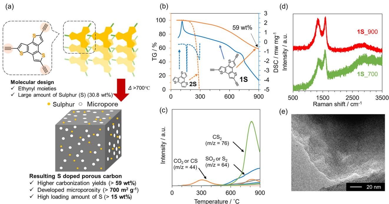
**Fig. 2** (a) Molecular design of the precursor and the schematic synthetic strategy for highly S-doped porous carbons. (b) TG-DSC profiles for **1S** (solid lines) and **2S** (dashed lines) and (c) the corresponding MS spectra for **1S**. (d) Raman spectra of **1S\_700** and **1S\_900**. (e) TEM image of **1S\_900**.
