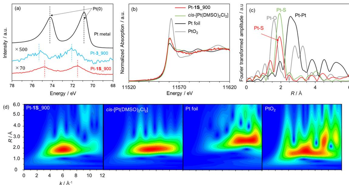
**Fig. 5** (a) Pt 4f XPS spectra of Pt-1S\_900, Pt-3\_900, and Pt metal. (b) Pt L<sub>3</sub>-edge XANES spectra and (c) Fourier transforms of  $k^3$ -weighted EXAFS oscillations for Pt-1S\_900, *cis*-[Pt(DMSO)<sub>2</sub>Cl<sub>2</sub>], Pt foil, and PtO<sub>2</sub>. (d) Wavelet transforms of Pt-1S\_900, *cis*-[Pt(DMSO)<sub>2</sub>Cl<sub>2</sub>], Pt foil, and PtO<sub>2</sub>.
