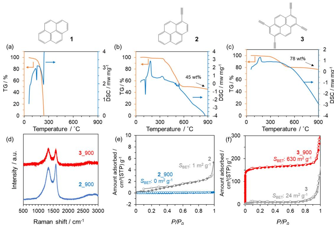
**Fig. 1** TG-DSC profiles of (a) 1, (b) 2 and (c) 3. (d) Raman spectra of 2\_900 and 3\_900. N<sub>2</sub> adsorption/desorption isotherms of (e) 2 and 2\_900, and (f) 3 and 3\_900.
