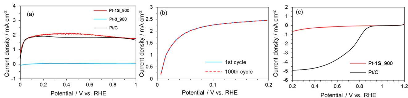
**Fig. 6** (a) Polarization curves for the HOR of Pt-1S<sub>900</sub>, Pt-3<sub>900</sub> and Pt/C under a H<sub>2</sub> flow. (b) Polarization curves for the HOR of Pt-1S<sub>900</sub> for the 1st and 100th cycle. (c) Polarization curves for the ORR of Pt-1S<sub>900</sub> and Pt/C.
