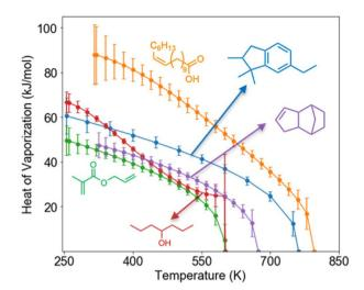
Fig. 2 Heat of vaporization of five example molecules in the NIST-WTT database.
