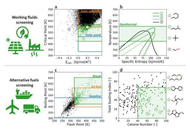
Fig. 8 Application of the GAT model for working fluid and alternative fuels screening. (a) Distribution of  $\sim$ 27 000 organic molecules on  $T_{\rm C}$ – $\xi$  axis, (b) T–s curve of four different working fluids with varying  $T_{\rm C}$  and  $\xi$ , (c) distribution of  $\sim$ 1300 saturated ethers on  $T_{\rm B}$ –FP axis, and (d) sub-screening based on YSI and CN.
