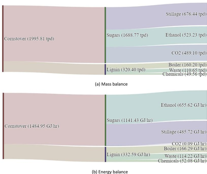
Fig. 4 (a) Mass balance and (b) Energy balance for converting corn stover to sugars followed by ethanol, and lignin conversion to chemicals.
