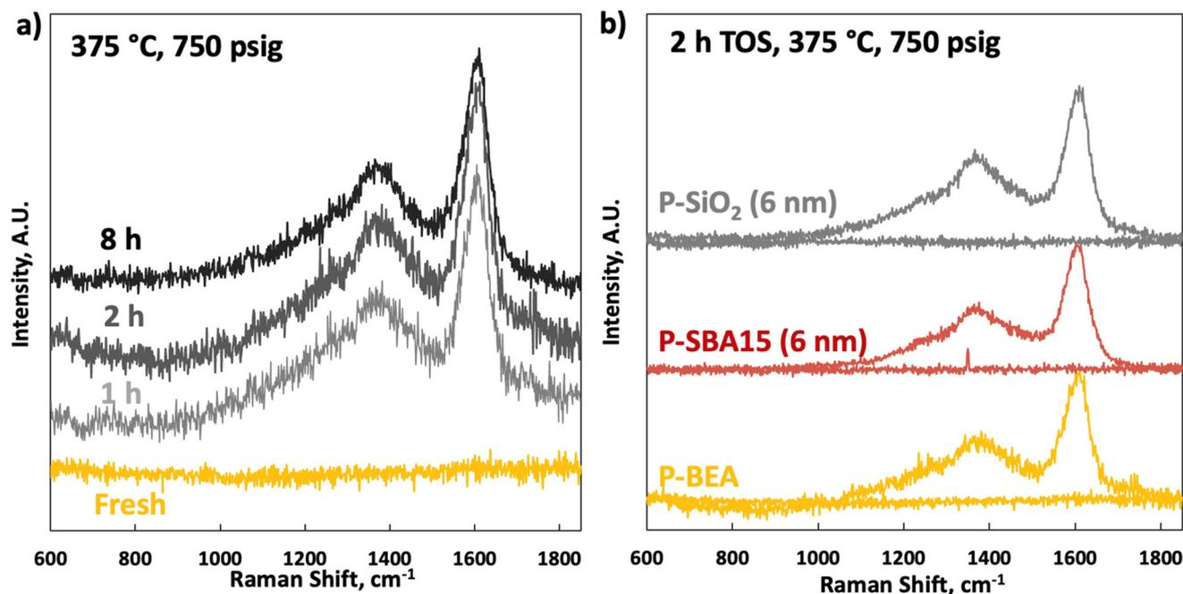
**Fig. 9** Raman spectra of (a) fresh P-BEA(25) and after 1, 2, and 8 h time on stream; and (b) fresh P-BEA, P-SBA-15 (6 nm mesopores) and P-SiO<sub>2</sub> (6 nm mesopores) at Si/P = 25 loading, and after 2 h time on stream. Conditions: 375 °C, 20 wt% DMF in *n*-heptane, 750 psig, 0.025 mL min<sup>-1</sup>, 10 sccm gas feed, 0.5 g of 150–250 μm pellets, 1/WHSV of 2.5 h, 0.01 g catalyst taken out at each sampling point.
