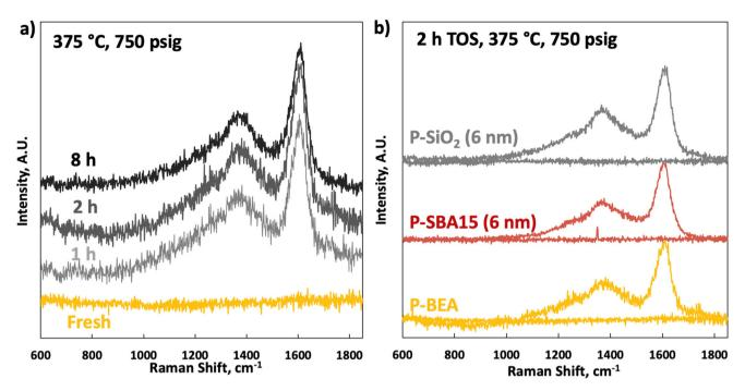
Fig. 9 Raman spectra of (a) fresh P-BEA(25) and after 1, 2, and 8 h time on stream; and (b) fresh P-BEA, P-SBA-15 (6 nm mesopores) and P-SiO<sub>2</sub> (6 nm mesopores) at Si/P = 25 loading, and after 2 h time on stream. Conditions: 375 °C, 20 wt% DMF in n-heptane, 750 psig, 0.025 mL min<sup>-1</sup>, 10 sccm gas feed, 0.5 g of 150-250 µm pellets, 1/WHSV of 2.5 h, 0.01 g catalyst taken out at each sampling point.
