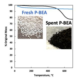
Fig. 8 Thermogravimetric analysis (TGA) of fresh and spent P-BEA(25). 20 wt% DMF in feed. Catalyst after10 h overall TOS exposed between 250  $^{\circ}$ C and 425  $^{\circ}$ C.
