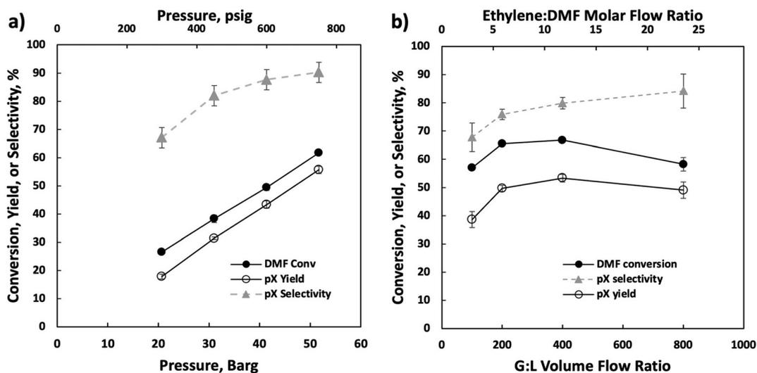
Fig. 3 Performance vs. flow reactor pressure (a) and gas : liquid feed ratio (b). Conditions: 375 °C, 20 wt% DMF in *n*-heptane feed, 0.025 mL min<sup>-1</sup> liquid feed. Only the gas flow rate was varied in changing the gas-to-liquid (G : L) ratio.
