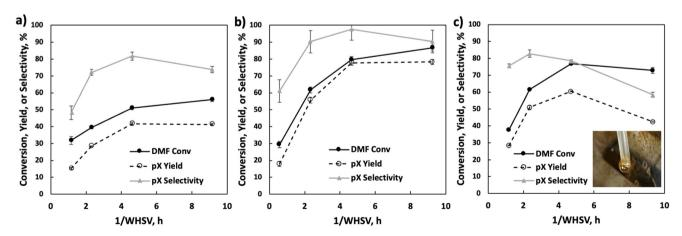
Fig. 5 Reactor performance at various 1/WHSVs at 350 °C (1.15 h, 2.31 h, 4.61 h, and 9.15 h, panel a), 375 °C (0.57 h, 2.33 h, 4.66 h, and 9.24 h, panel b), and 400 °C (1.18 h, 2.35 h, 4.70 h, and 9.33 h, panel c). Conditions: 750 psig back pressure, 0.5 g P-BEA(25), 20 wt% DMF feed; 0.025 mL  $min^{-1}$  liquid flow rate.
