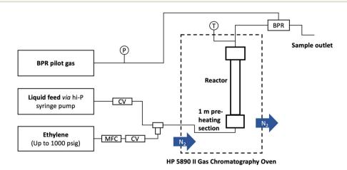
Fig. 2 Flow chemistry setup.
