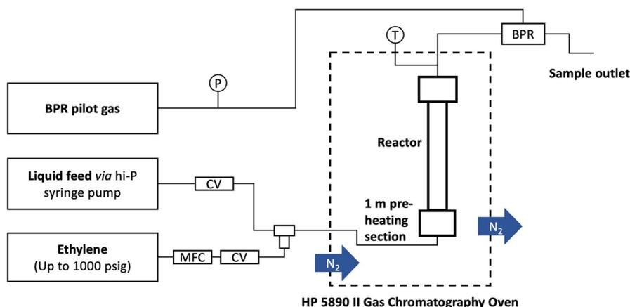
Fig. 2 Flow chemistry setup.
