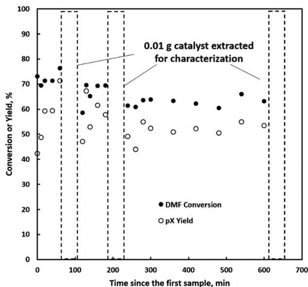
**Fig. 7** Time-on-stream (TOS) performance of P-BEA(25) with small portions of the catalyst taken out at 1, 2, and 8 h. The time after catalyst sampling was set to 50 min for easy visualization. Conditions: 375 °C, 20 wt% DMF in *n*-heptane, 750 psig, 0.025 mL min<sup>-1</sup>, 10 sscm gas feed, 0.5 g 150–250 μm pellets, 0.01 g catalyst taken out at each instant.
