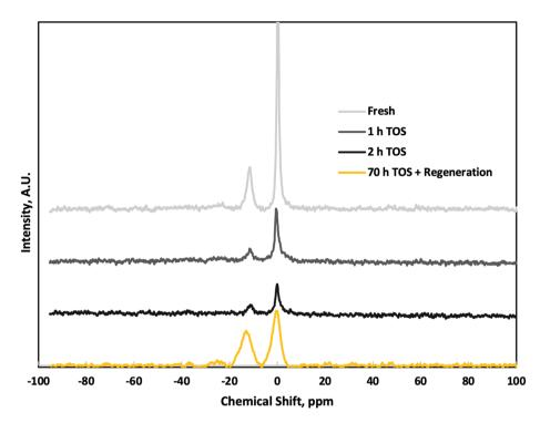
Fig. 10  $^{31}$ P NMR spectra of fresh P-BEA (25) and post-reaction at 1 and 2 h TOS, and post-reaction after *in situ* regeneration following ~70 hours of continuous operation. 375 °C, 20 wt% DMF in *n*-heptane, 750 psig, 0.025 mL min<sup>-1</sup>, 10 sccm gas feed, 0.5 g 150–250  $\mu$ m pellets, 0.01 g catalyst sampled at each TOS.
