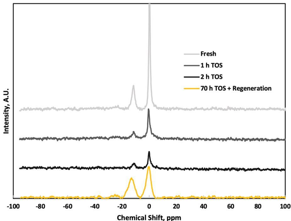
**Fig. 10**  $^{31}\text{P}$  NMR spectra of fresh P-BEA (25) and post-reaction at 1 and 2 h TOS, and post-reaction after *in situ* regeneration following  $\sim 70$  hours of continuous operation.  $375^\circ\text{C}$ , 20 wt% DMF in *n*-heptane, 750 psig,  $0.025\text{ mL min}^{-1}$ , 10 sccm gas feed, 0.5 g 150–250  $\mu\text{m}$  pellets, 0.01 g catalyst sampled at each TOS.
