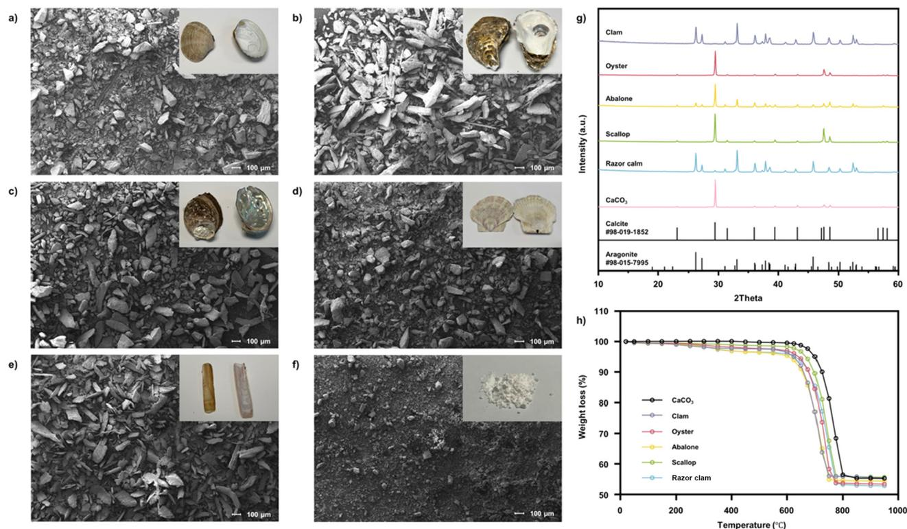
**Fig. 2** (a–f) Photos and SEM images (100×) of (a) clam; (b) oyster; (c) abalone; (d) scallop; (e) razor clam; and (f) calcium carbonate. (g) XRD patterns of different seashells and pure calcium carbonate. (h) TG curves of different seashells and pure calcium carbonate.
