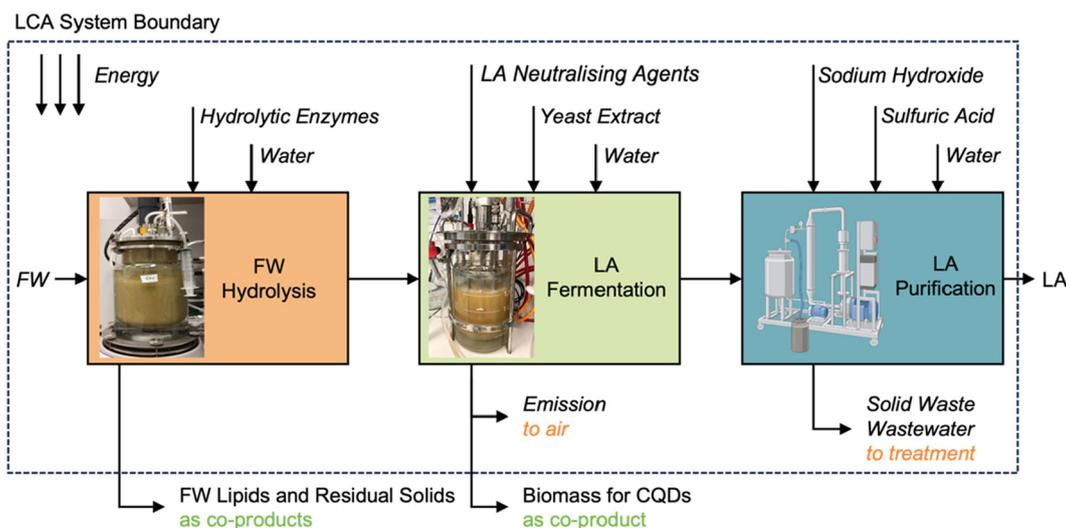
**Fig. 1** System boundary diagram. Italics indicate the connection to background LCI databases. FW: food waste. LA: lactic acid. LA neutralising agents: NaOH, shell,  $\text{Ca}(\text{OH})_2$ . Glucoamylase is used in FW hydrolysis in the simulation process.
