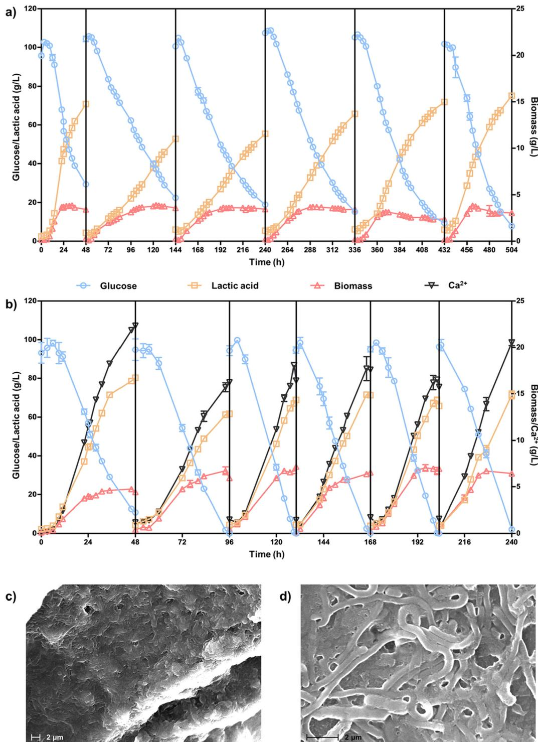
**Fig. 5** (a) Lactic acid fermentation in *is*FBB using FWH medium and 10 M NaOH as the pH control. (b) Lactic acid fermentation in *is*FBB using FWH medium and fine shell powder as the pH control. (c) SEM image of the surface of sugarcane bagasse (5000 $\times$ ). (d) SEM image of immobilised cells (20 000 $\times$ ).
