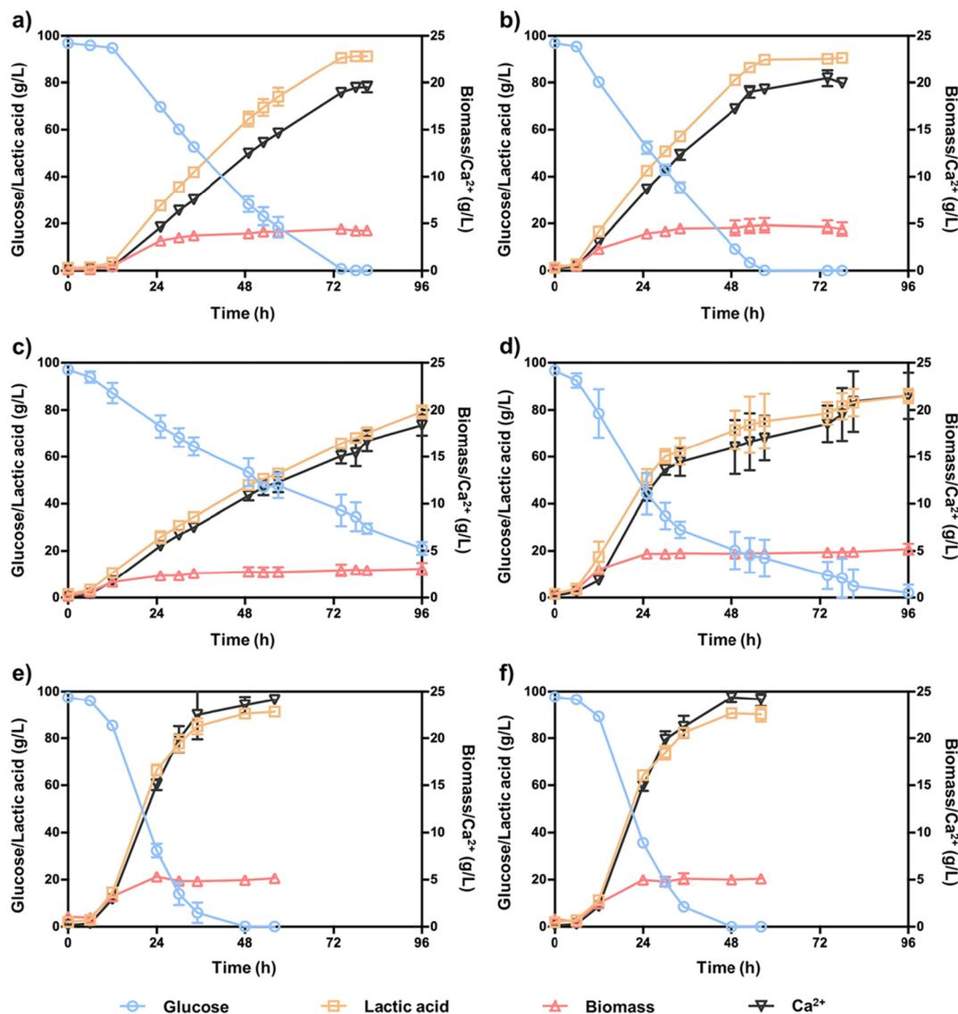
**Fig. 3** Lactic acid fermentation in shake flasks using MRS and FWH medium with different forms of seashell as the acid neutraliser. (a) MRS medium + shell piece; (b) MRS medium + shell powder; (c) FWH medium + shell piece; (d) FWH + shell powder; (e) FWH medium + fine shell powder; and (f) FWH medium + CaCO<sub>3</sub>.
