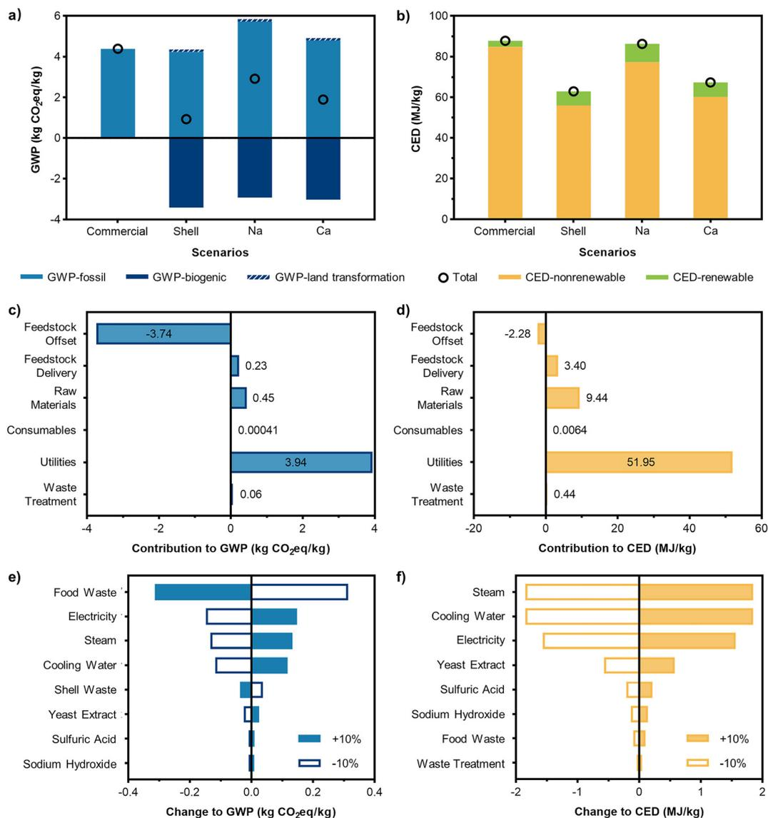
**Fig. 6** Summary of global warming potential (GWP) and cumulative energy demand (CED) results. (a) GWP of three scenarios in comparison with commercial lactic acid. (b) CED of three scenarios in comparison with commercial lactic acid. (c) Breakdown of GWP in Scenario Shell. (d) Breakdown of CED in the Scenario Shell. (e) Sensitivity analysis of GWP in Scenario Shell. (f) Sensitivity analysis of CED in Scenario Shell.
