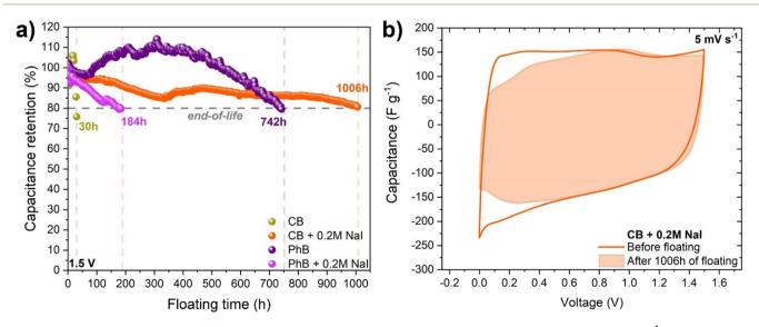
Fig. 5 (a) Capacitance retention of YP50F-based ECs operating in citrate buffer and phosphate buffer with/without 0.2 mol L<sup>-1</sup> Nal additive during floating test (at 1.5 V). Cyclic voltammograms for ECs operating in (b) citrate buffer + 0.2 mol L<sup>-1</sup> Nal before and after 1006 h floating test.
