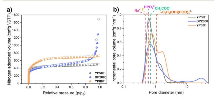
Fig. 1 (a) Nitrogen adsorption/desorption isotherms at 77 K; (b) pore-size distributions of YP50F, BP2000, YP80F activated carbons and pore diameters of selected solvated ions.
