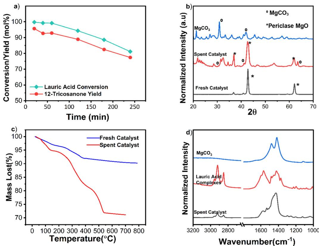
Fig. 4 (a) TOS data of MgO. Reaction conditions: lauric acid flowrate: 0.1 g min<sup>-1</sup>, WSHV 0.1 min<sup>-1</sup>, 1 g MgO catalyst, and a reaction temperature 365 °C. (b) XRD spectra of fresh, spent, and regenerated catalyst (calcined at 600 °C in air for 2 h). (c) TGA data of the spent and fresh catalysts in N<sub>2</sub> from 20–700 °C at a ramp rate of 20 °C min<sup>-1</sup>. (d) FTIR spectra of the spent catalyst compared with pure MgCO<sub>3</sub> and lauric acid complexes.
