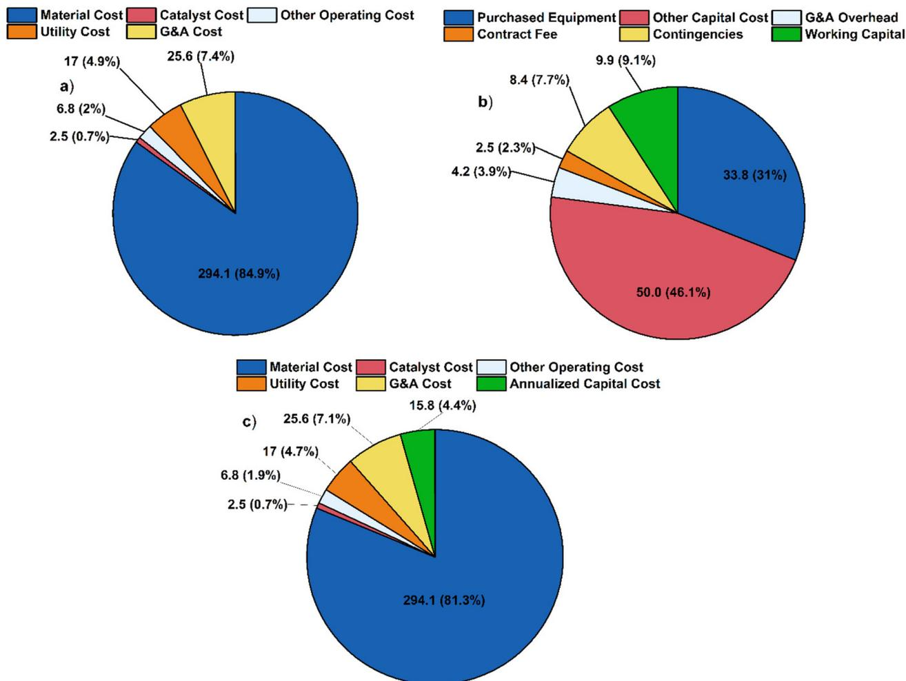
**Fig. 9** (a) Operating cost breakdown. Graph labels refer to cost in million \$ per year along with the percentage of total operating cost. (b) Capital cost breakdown, in millions of dollars. (c) Total cost breakdown, numbers are presented in million \$ per year for the base case scenario with 12-tricosanone produced through self-ketonization of lauric acid.
