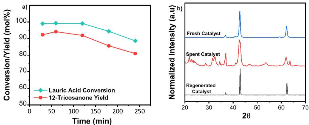
Fig. 5 (a) Activity of 1 g of regenerated catalyst, WSHV 0.1 min<sup>-1</sup>, reaction temperature 365 °C. (b) XRD spectra of fresh, spent, and regenerated catalysts.
