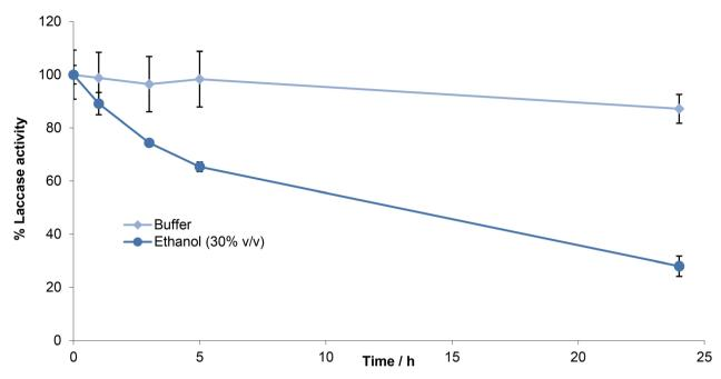
Fig. 4 Residual activity of laccase after incubation in the presence of ethanol.
