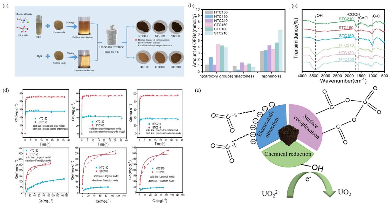
**Fig. 8** (a) Synthesis schematic of HTCs and STCs. (b) Contents of oxygen-containing functional groups of HTCs and STCs. (c) FTIR spectra. (d) The adsorption kinetics and adsorption isotherms of HTCs and STCs. (e) The adsorption mechanism of U(vi) on STCs.<sup>23</sup> With permission. Copyright 2023 Elsevier.
