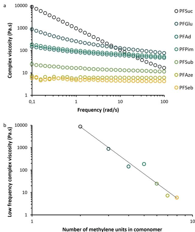
**Fig. 10** (a) Complex viscosity versus angular frequency and (b) low shear viscosity ( $0.1 \text{ rad s}^{-1}$ ) versus the number of methylene units in the comonomer of the enzymatically produced BHMf-based polyesters, measured at a constant temperature at  $30 \text{ }^\circ\text{C}$  above the melting temperature. Equation trendline:  $y = 3.4 \times 10^5 x^{-5.3}$ ,  $R^2 = 0.9994$ .
