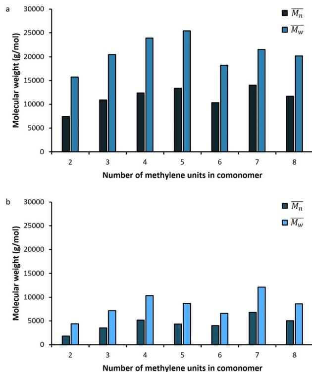
**Fig. 3** Number average molecular weight ( $\overline{M}_n$ ) and weight average molecular weight ( $\overline{M}_w$ ) of BHMf-based polyesters containing different numbers of methylene units in the comonomer segment, catalyzed by either iCALB (a) or DBTO (b).
