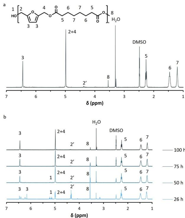
Fig. 2 (a) Normalized <sup>1</sup>H-NMR spectrum of poly(2,5-furandimethylene suberate) (PFSub) in DMSO-*d*<sub>6</sub>, (b) <sup>1</sup>H-NMR spectra of PFSub during iCALB-catalyzed polycondensations at different times.
