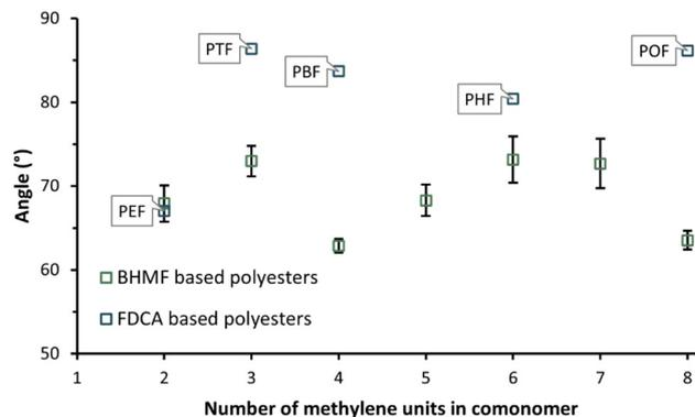
**Fig. 9** Average water contact angle of the enzymatically produced BHMf-based polyester discs (this work) and FDCA-based polyesters: poly(ethylene 2,5-furandicarboxylate) (PEF), poly(trimethylene 2,5-furandicarboxylate) (PTF), poly(butylene 2,5-furandicarboxylate) (PBF), poly(hexylene 2,5-furandicarboxylate) (PHF), and poly(octylene 2,5-furandicarboxylate) (POF), obtained from.<sup>54</sup>
