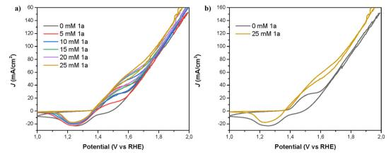
Fig. 6 (a) Cyclic voltammetries for the oxidation of 1a (0-25 mM), using NiNF as the working electrode, Pt wire as the counter electrode and Ag/ AgCl as the reference (RHE potential scale), in 0.5 M KOH as the electrolyte at 5 mV s<sup>-1</sup> scan. (b) Zoom cyclic voltammetries for the oxidation of 1a (0 and 25 mM).
