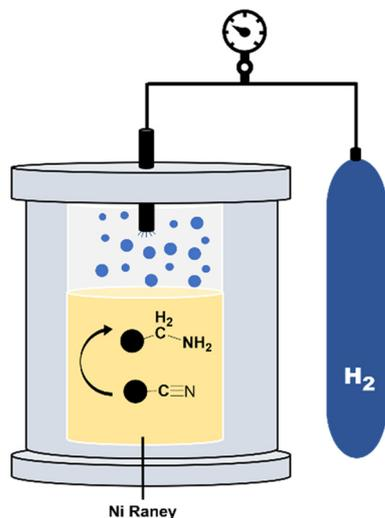
Fig. 10 Scheme of a high-pressure reactor.
