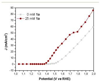
Fig. 7 J-V curves obtained during IS measurement of NiNF electrodes in a 0.5 M KOH aqueous solution with and without 1a.
