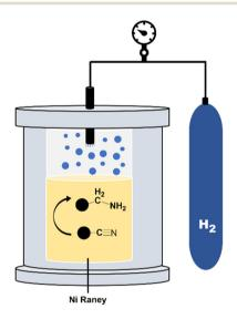
Fig. 10 Scheme of a high-pressure reactor.
