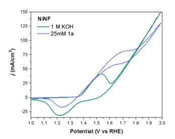
Fig. 3 Comparison of cyclic voltammetry curves of NiNF, in 20 mL of 1 M KOH, with and without 1a.
