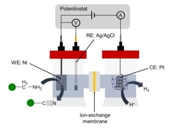
Fig. 4 Scheme of a two-compartment cell.
