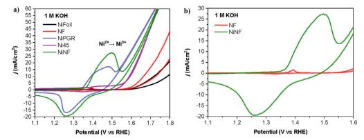
Fig. 2 (a) Cyclic voltammetry curves at a scan rate of 10 mV s<sup>-1</sup> of all Ni electrodes in 20 mL of 1 M KOH. (b) Details of (a) for a better comparison of NF and NiNF cyclic voltammetry curves.
