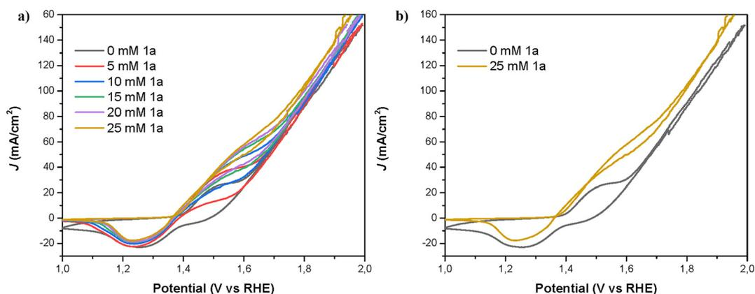
**Fig. 6** (a) Cyclic voltammograms for the oxidation of **1a** (0–25 mM), using NiNF as the working electrode, Pt wire as the counter electrode and Ag/AgCl as the reference (RHE potential scale), in 0.5 M KOH as the electrolyte at 5 mV s<sup>-1</sup> scan. (b) Zoom cyclic voltammograms for the oxidation of **1a** (0 and 25 mM).
