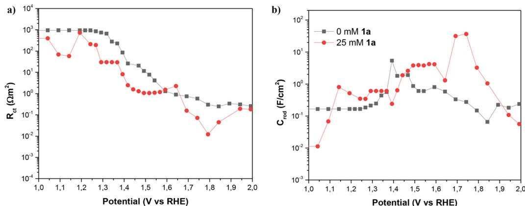
Fig. 9 (a) Charge transfer resistance and (b) capacitance of NiNF as a function of the potential vs. RHE with and without **1a**, in 0.5 M KOH. Figures (a) and (b) hold the same legend.
