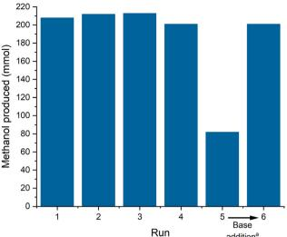
Fig. 4 Amount of methanol produced and theoretical yield in the catalyst recycling experiment in the hydrogenation of CO. Conditions: CO (20 bar), H<sub>2</sub> (100 bar), Mn-1 (92 μmol), NaOMe (4.65 mmol, 50 eq.), 1-dodecanol (70 ml), 150 °C, 4 h, 300 mL reactor. (a) Addition of NaOMe (4.65 mmol) in 1-dodecanol (10 ml)
