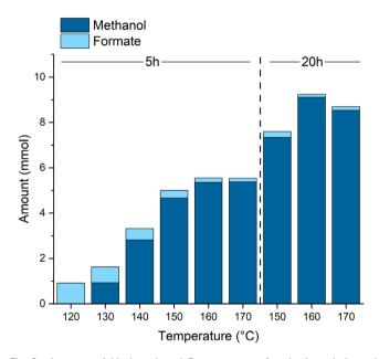
Fig. 2 Amount of Methanol and Formate ester (total of methyl- and dodecylformate) at various temperatures and reaction times. Conditions: CO (10 bar), H $_2$  (50 bar), Mn-1 (2  $\mu$ mol), NaOMe (50  $\mu$ mol), 25% methanol in 1-dodecanol (1.5 ml), T, t, 20 mL autoclave.
