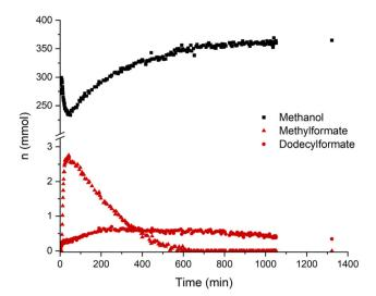
Fig. 3 Product and intermediate time profile based  $^1H$  NMR measurements with internal standard THF. Conditions: CO (8 bar),  $H_2$  (32 bar), Mn-1 (48  $\mu$ mol), NaOMe (2.4 mmol), 25% methanol in 1-dodecanol (25 ml), 150 °C, 280 mL reactor.  $\delta=3.33$  (s, 3 H,  $H_3C$ -OH (methanol)), 8.02 (s, 1 H, OOCH (methyl formate)), 8.53 (m, 1 H, OOCH (dodecyl formate)) ppm.
