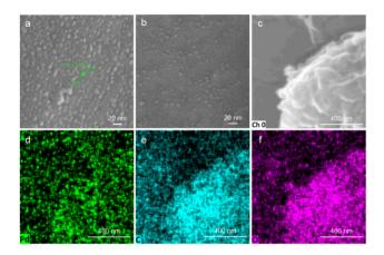
Fig. 2 Scanning electron microscopy images of the Pd/ $\alpha$ -CD (a) after the first run and (b) after the fifth run. (c-f) EDS-SEM images of the Pd/ α-CD after the fifth run.
