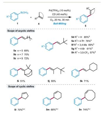
Scheme 2 Substrate scope for the unfunctionalized aliphatic olefins.<sup>a</sup> Reaction conditions: 1 (0.5 mmol), 4 (0.5 mmol), Pd(TFA)<sub>2</sub> and  $\alpha$ -CD (40 mol%) were placed in a stainless-steel vessel with two stainless-steel balls ( $\varnothing$  = 1.2 cm) milling at 20 Hz for 30 min under an oxygen atmosphere. Isolated yields. <sup>b</sup> Two equiv. of olefins were added. <sup>c</sup>  $\beta$ -CD was used instead of  $\alpha$ -CD.
