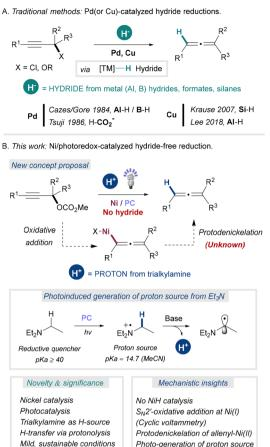
Fig. 1 Synthetic methods for allenes involving transition metal (TM)catalyzed reduction of propargyl electrophiles.
