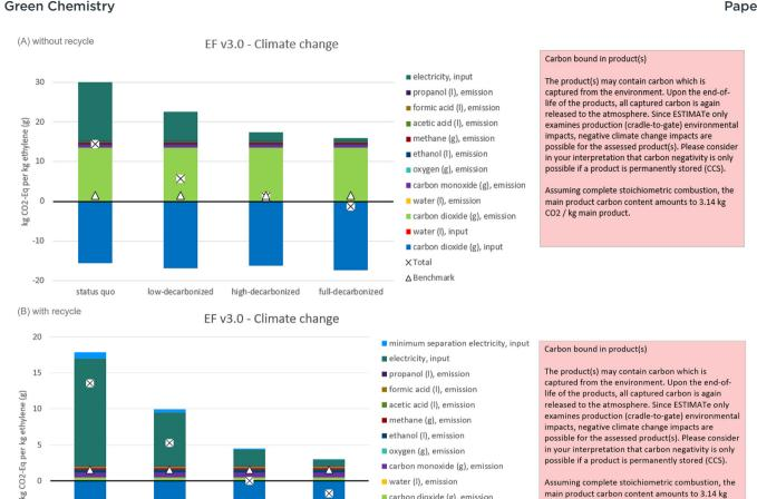
Fig. 5 Climate Change Impact of laboratory-scale electrochemical CO2 reduction to ethylene in the ESTIMATe tool. (A) Without recycle of unreacted CO2, (B) including a recycle of unreacted CO2. Note the different scales of the y-axes. The different bars correspond to the different background system scenarios defined in section 2.4.
