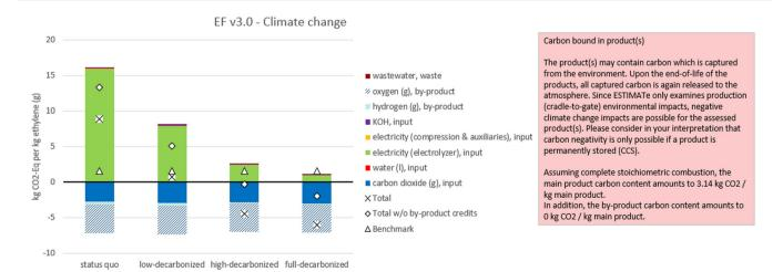
Fig. 6 Climate Change Impact of process-design-scale electrochemical CO<sub>2</sub> reduction to ethylene calculated by the ESTIMATe tool. The different bars correspond to the different background system scenarios defined in section 2.4.
