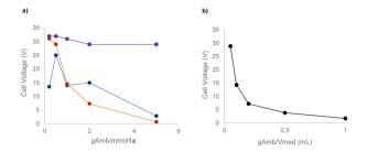
Scheme 1 Mass/volume and mass/mmol plot to identify the suitability of the solid electrolyte at 6 mA constant current using a C anode and an Al cathode. (a) Grams of Amb-400-Cl/mmol of the 1a ratio over the cell voltage potential plot; blue line: in 2 mL of acetonitrile; red line: in 5 mL of acetonitrile; purple line: in 10 mL of acetonitrile. (b) Grams of Amb-400-Cl/mL of the acetonitrile ratio over the cell voltage potential plot.
