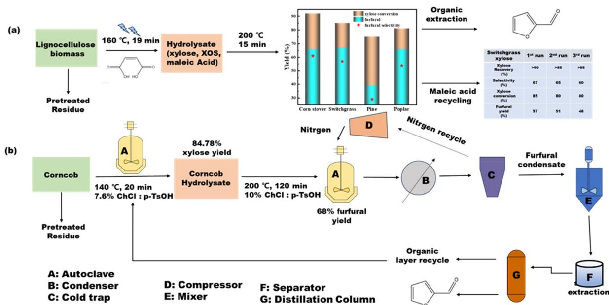
Fig. 9 Two-step process for furfural production *via* maleic acid (a) and ChCl : p-TsOH (b).<sup>119,121</sup>
