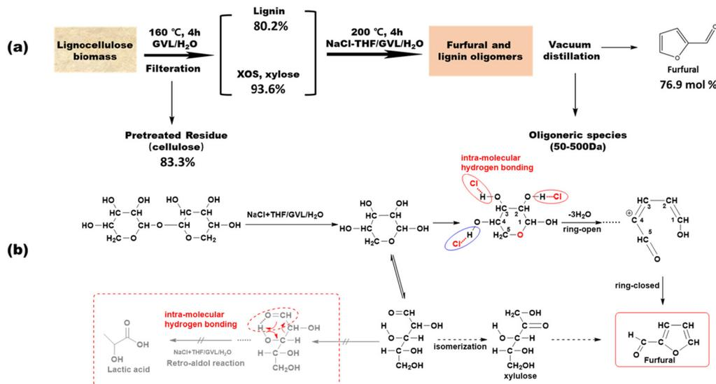
Fig. 11 The two-step process (a) and proposed mechanism of NaCl+THF/GVL/H<sub>2</sub>O system (b) for furfural production.<sup>132</sup>
