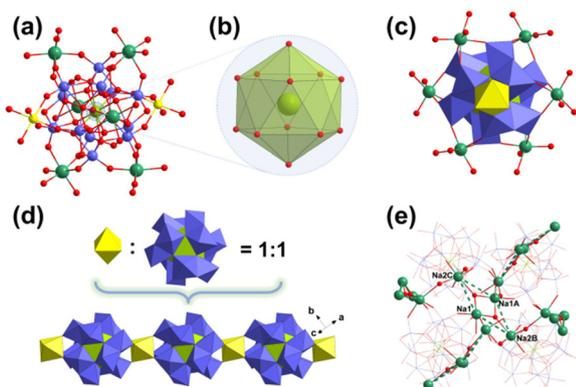
**Fig. 1** (a) Ball-and-stick view of the  $\{FeUMo_{12}\}$  unit; (b) the coordination environment of U1; (c) the six disordered Na ions coordinated with one center  $\{FeUMo_{12}\}$  unit; (d) schematic diagram of the  $\{FeUMo_{12}\}_n$  1D chain; (e) the connection modes of the tetranuclear Na–H<sub>2</sub>O clusters. Color codes: Fe(II), yellow; U(IV), light green; Mo, blue; Na, green; O, red.
