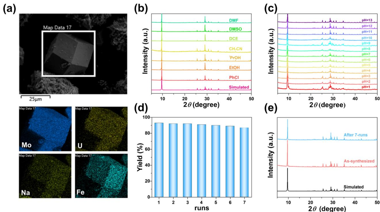
**Fig. 3** (a) The EDS mapping of metal elements in FeUMo; (b) the PXRD patterns of NiUMo after being heated in different organic solvents for one day; (c) the PXRD patterns of NiUMo after being soaked in water solutions with different pH values for one day; (d) the cyclic yields of NiUMo; (e) the PXRD patterns of NiUMo after 7-cycles catalytic reactions.
