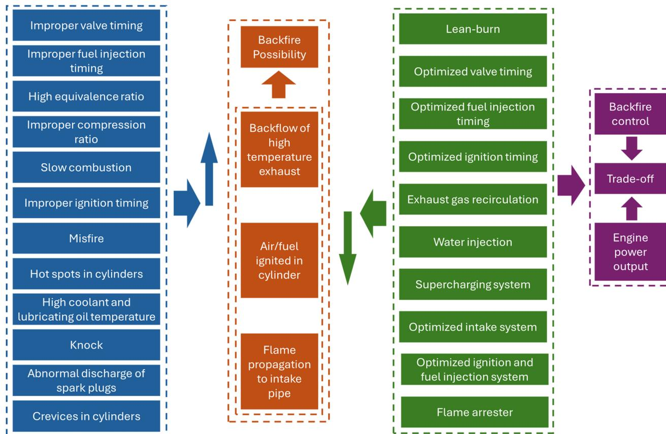
Fig. 15 Control measures for various factors of backfire in hydrogen engines. Re-drawn from ref. 32.
