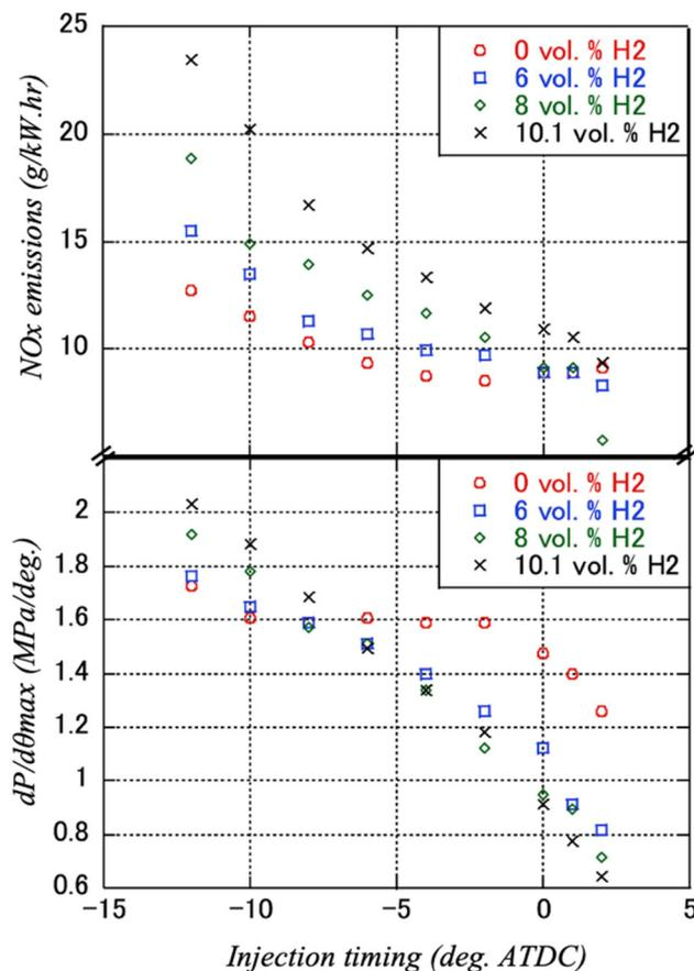
Fig. 11 Variations of NO<sub>x</sub> and  $dP/d\theta_{max}$  with diesel fuel injection timing for different hydrogen fractions. Re-drawn from ref. 110 and 111.
