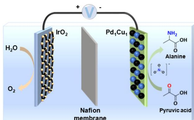
Fig. 7 Electrocatalytic conversion of pyruvic acid and nitrate into alanine. Adapted and modified with permission from ref. 58. Copyright 2023 John Wiley and Sons.
