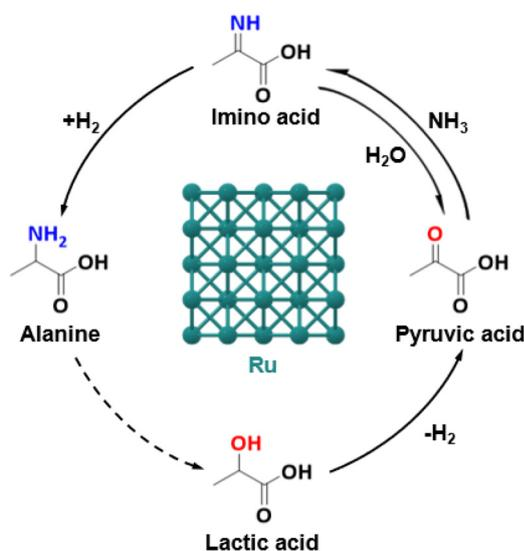
Fig. 5 Thermocatalytic conversion of lactic acid and  $\text{NH}_3$  into alanine using a Ru-based catalyst.<sup>11,49,52</sup>
