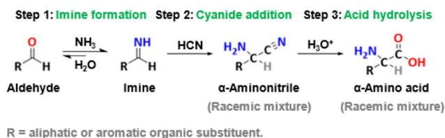
Fig. 2 The Strecker synthesis of  $\alpha$ -amino acids.<sup>3,31</sup>
