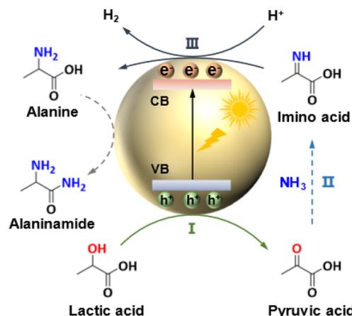
Fig. 6 Photocatalytic conversion of lactic acid and  $\text{NH}_3$  into alanine.<sup>13</sup>
