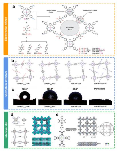
Fig. 8 Schematic illustration of the side chain modulation of COFs. (a) Design of cobalt-porphyrin derived covalent organic frameworks; <sup>117</sup> (b) schematics and (c) images of contact angles of crosslinked metalloporphyrin networks with different electron-flow and mass-transport interfaces; <sup>119</sup> (d) synthesis of phenazine-linked COPc-based COFs; <sup>120</sup> (e) synthesis of phenazine-linked NiPc-based COFs with *tert*-butyl groups. <sup>121</sup>
