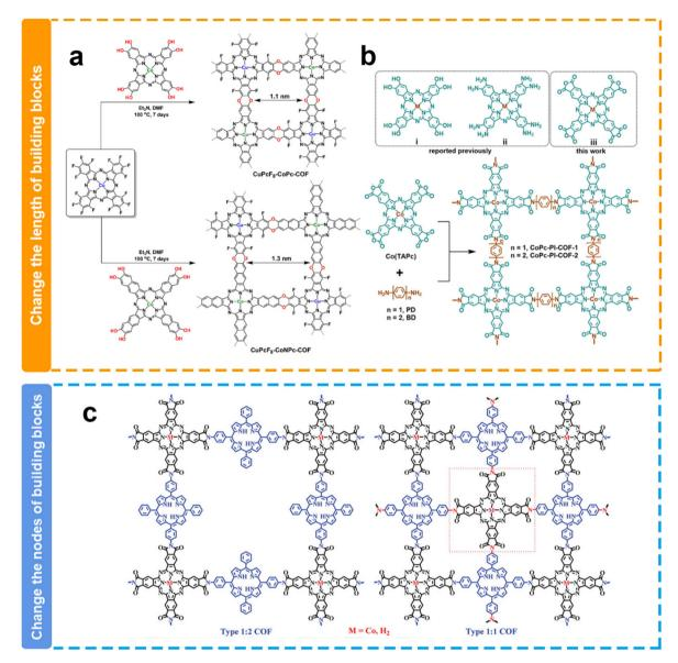
Fig. 9 Schematic illustration of the pore size modulation of COFs. (a and b) Schematic illustration of the modulation of the COF pore size *via* length building blocks; 124,125 (c) schematic illustration of the modulation of the COF pore size *via* the nodes of building blocks.
