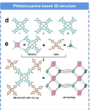
**Fig. 10** Schematic illustration of the synthesis of different 3D COFs and their performance. (a) Schematic illustration of prepare porphyrin-based 3D COF; (b) LSV curves and (c) FE of porphyrin-based 3D COF; (d) Different kinds of phthalocyanine building blocks, (e) Schematic illustration of the preparation of phthalocyanine-based 3D COF. 129
