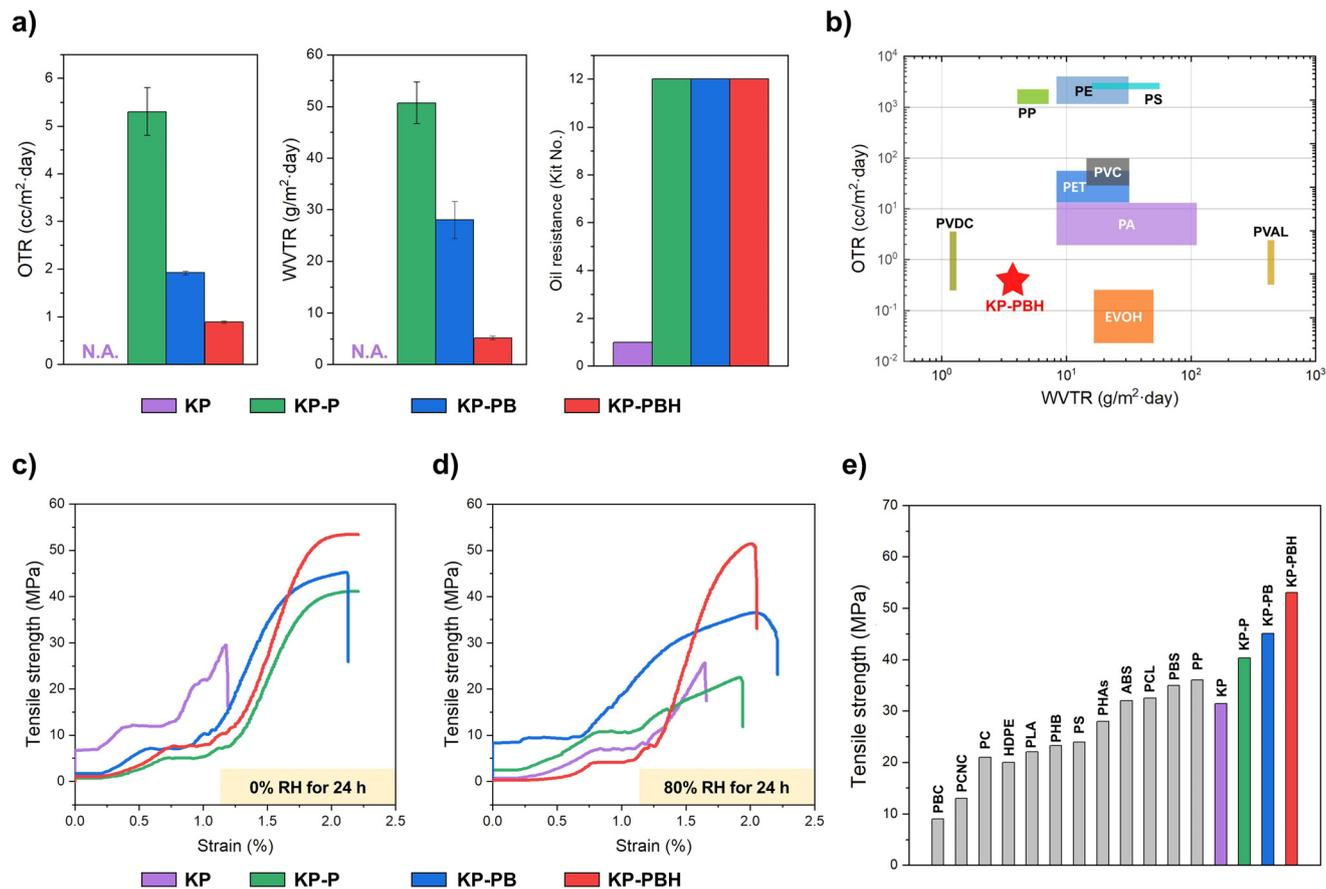
**Fig. 3** (a) Oxygen transmission rate (OTR), water vapor transmission rate (WVTR), and oil resistance of KP and coated papers (KP-P, KP-PB, and KP-PBH). (b) Comparative barrier properties of KP-PBH. (c and d) Tensile curves tested under dry and moist conditions. (e) Comparative tensile strength of commodity plastics and the coated papers. N.A.: not applicable.
