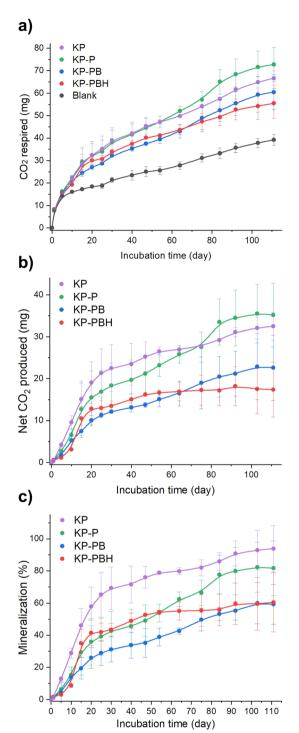
Fig. 4 Results of biodegradation test simulating marine environment employing respirometer. (a) Cumulative respired  $CO_2$ , (b) net  $CO_2$  produced, and (c) mineralization of KP, KP-P, KP-PB, and KP-PBH, calculated based on the difference in  $CO_2$  production between the samples and the blank (incubated without substrate) divided by theoretical  $CO_2$  production. Error bars are standard deviations of cumulative values (n = 2). The detailed description for calculation is in Text S1.†
