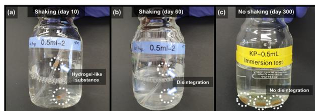
**Fig. 5** Photos of KP-PBH bioreactor showing the impact of mechanical stress on disintegration. KP-PBH after (a) 10 d and (b) 60 d of the biodegradation test using a respirometer where the bioreactors were shaken at 180 rpm. (c) KP-PBH after 300 d of immersion in the marine seawater and sediment mixture (i.e., no shaking).
