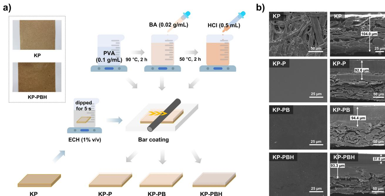
**Fig. 1** (a) Photos of KP and KP-PBH and the fabrication process of coated papers (KP-P, KP-PB, and KP-PBH). (b) SEM images of top-view and cross-section of coated papers. Scale bars are at the bottom right of each image.
