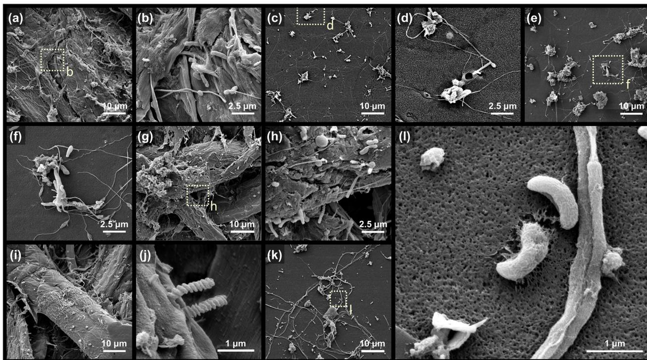
**Fig. 6** SEM images of surface morphology and microbes. (a and b) KP, (c and d) KP-P, (e and f) KP-PB, (g and h) KP-PB (uncoated side), (i and j) KP-PBH (uncoated side), and (k and l) KP-PBH after being immersed in seawater and sediment mixture for 60 d. The curved-rod bacteria assimilating the BA-crosslinked PVA coating are highlighted in (l). Dotted square region indicates the enlargement in the subsequent image. Scale bars are located at the bottom right of each image.
