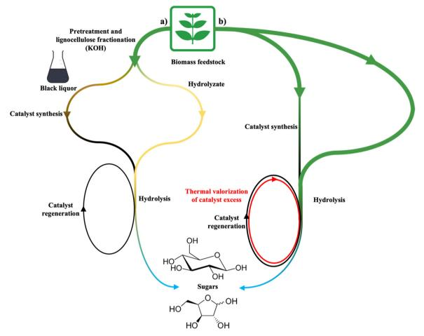
Fig. 7 BDC role in biomass valorisation according to the approaches followed by (a) Qi *et al.* (fractionated lignin-derived catalyst);<sup>176</sup> (b) Kobayashi *et al.* (biomass-derived catalyst with thermal valorisation of CM excess).<sup>177</sup>
