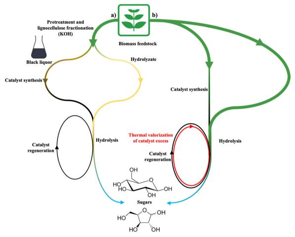
Fig. 7 BDC role in biomass valorisation according to the approaches followed by (a) Qi *et al.* (fractionated lignin-derived catalyst);<sup>176</sup> (b) Kobayashi *et al.* (biomass-derived catalyst with thermal valorisation of CM excess).<sup>177</sup>
