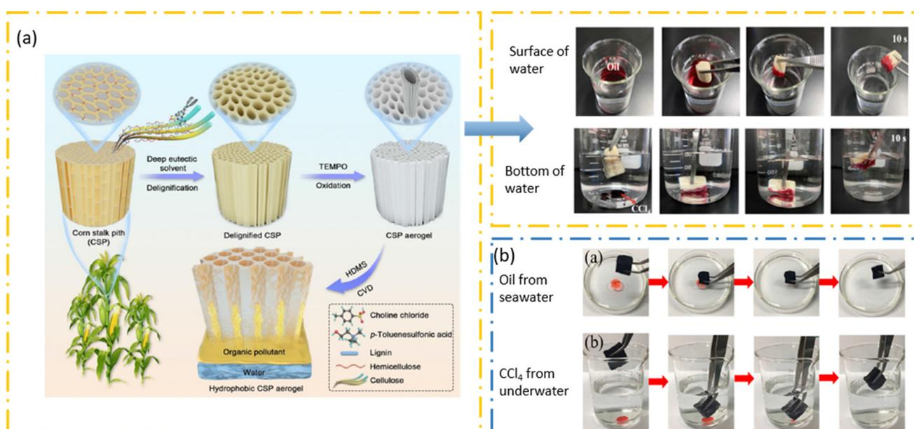
**Fig. 7** (a) Top-down approach for generating a hydrophobic aerogel from cornstalk pith that demonstrated a good oil/water separation capability.<sup>136</sup> Copyright 2023, Elsevier. (b) Absorption of oil from sea water and  $\text{CCl}_4$  from underwater using a carbon aerogel derived from DES-modified CNFs.<sup>135</sup> Copyright 2021, Elsevier.
