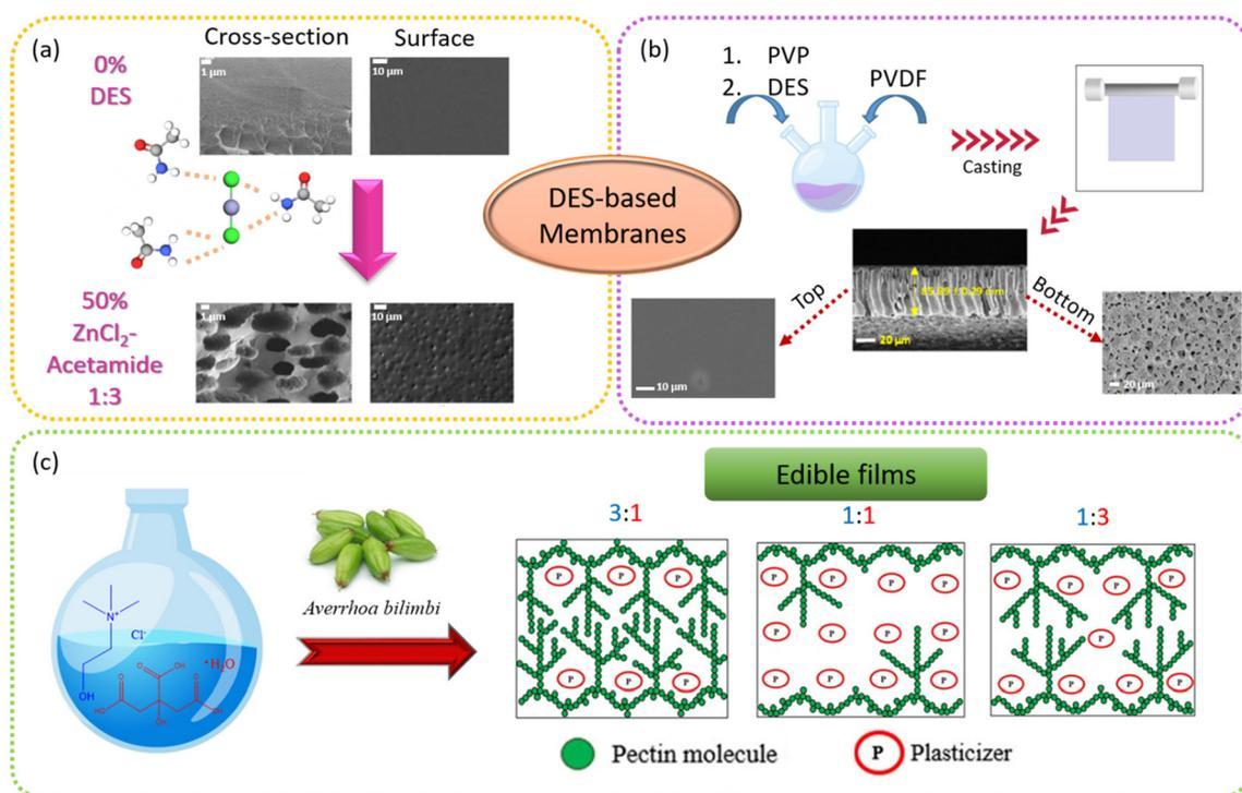
**Fig. 10** Illustration of the generation of porous membranes and their SEM images. (a) Polyamide-imide membranes before and after incorporation of ZnCl<sub>2</sub>:acetamide.<sup>164</sup> Copyright 2021, MDPI. (b) With non-ionic DES (*N*-methyl acetamide:*N*-methyl urea).<sup>165</sup> Copyright 2022, Elsevier. (c) Schematic illustration of the plasticization effect of edible films generated by *Averrhoa bilimbi* pectins with a DES.<sup>175</sup> Copyright 2020, Elsevier.
